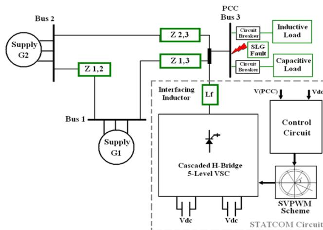
Figure 1. IEEE 3-Bus system with proposed STATCOM circuit
