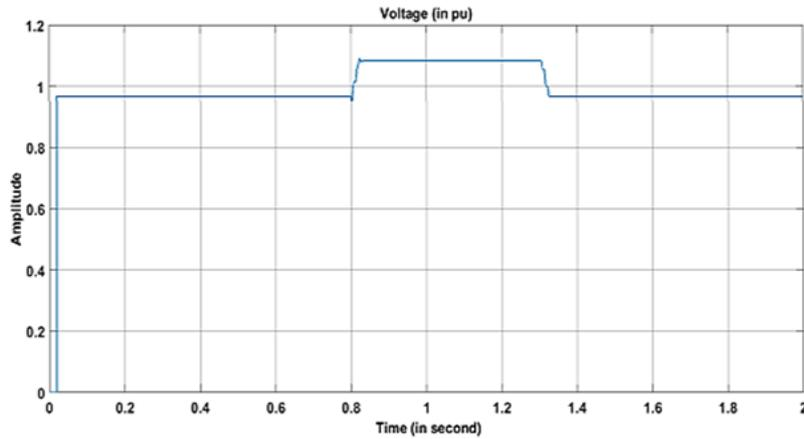
Figure 10. Voltage magnitude in the presence of voltage swell without the STATCOM
