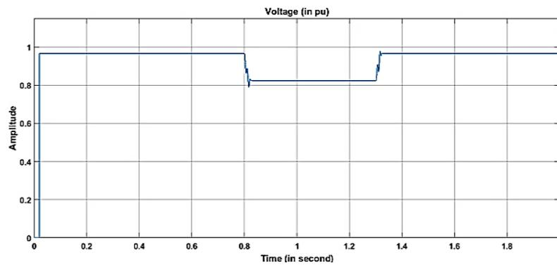
Figure 6. Voltage magnitude without the STATCOM when there is voltage sag
