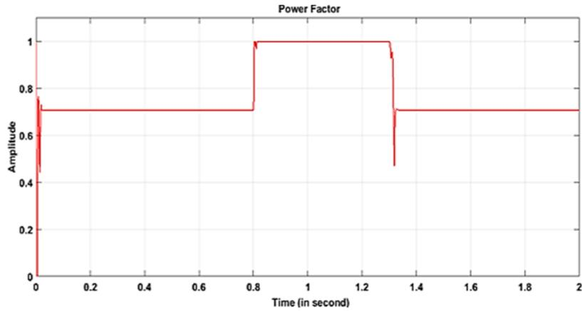
Figure 8. PF in the presence of voltage sag without the STATCOM
