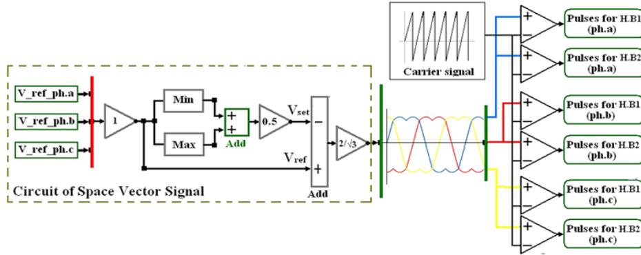
Figure 3. SVPWM scheme for cascaded 5-level VSC STATCOM
