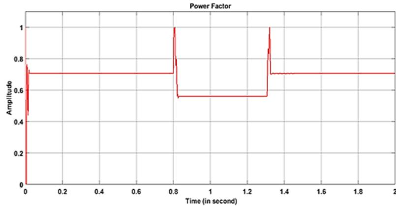
Figure 12. PF in the presence of voltage swell without the proposed STATCOM
