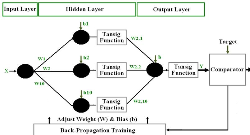
Figure 5. Structure of the NN controller
