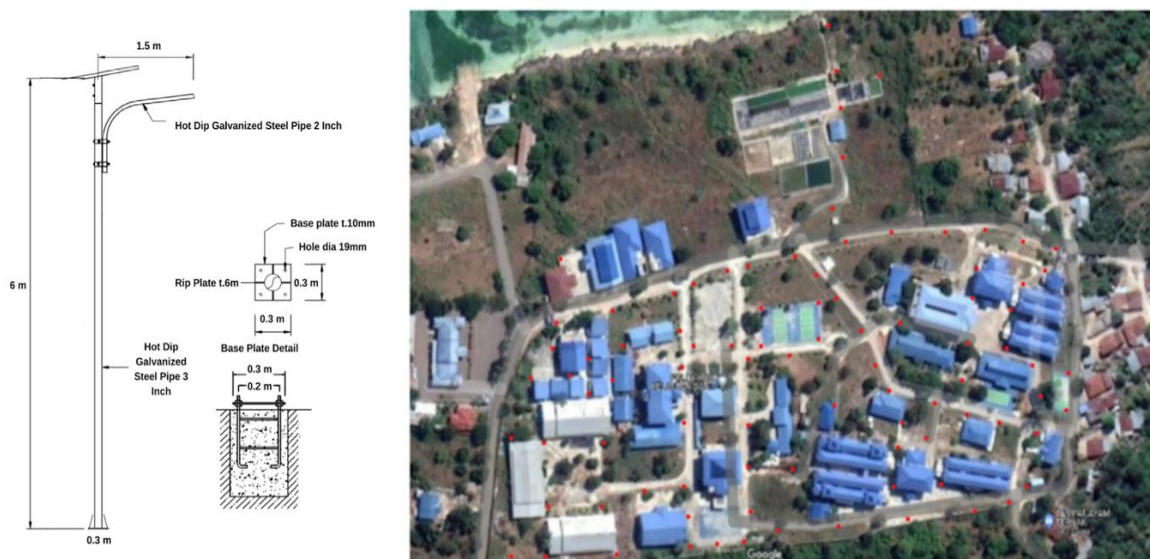
Figure 2. Design of a solar lighting system on campus
