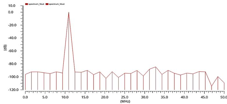
Figure 13. The output of the 2x-gain mode analyzed through a 64-point fast Fourier transform (FFT) to produce its spectrum
