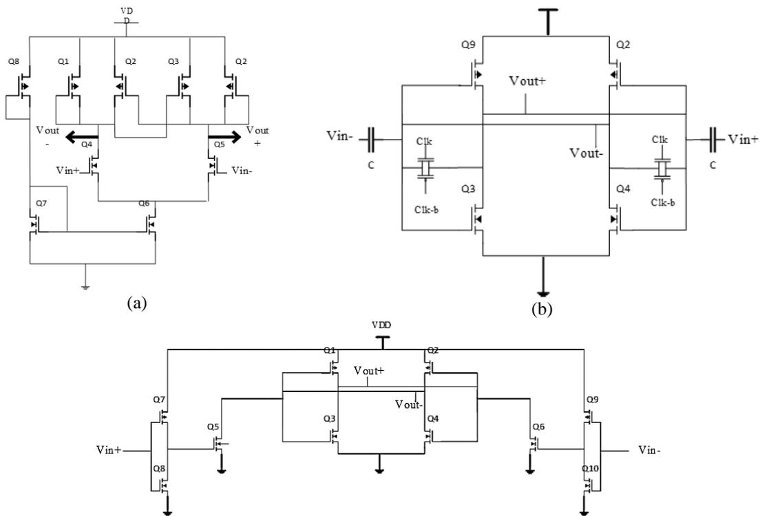
Figure 4. Blocks of the comparator: (a) preamp, (b) regenerative latch, and (c) RS-latch
