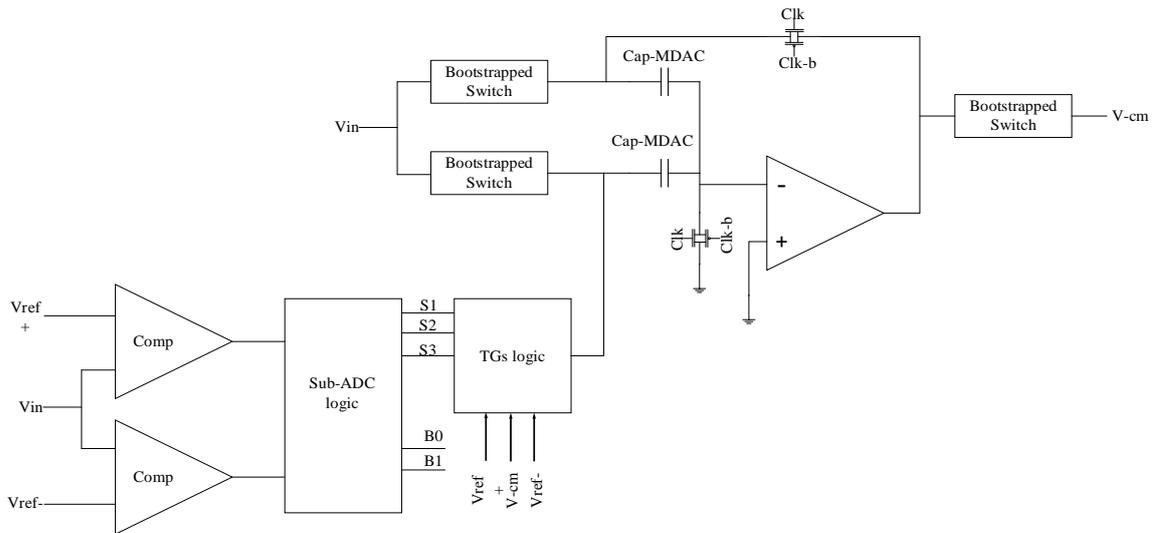
Figure 2. The 1.5-bit pipelined stage
