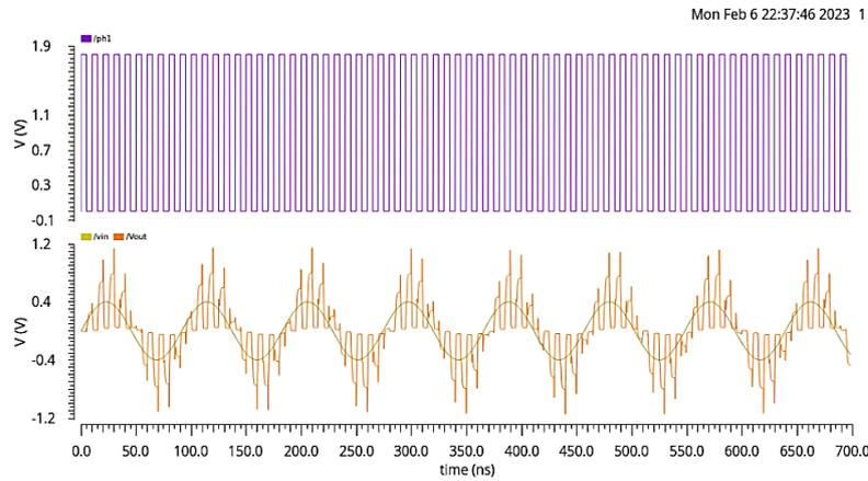
Figure 12. Transient simulation waveforms in 2x-gain mode
