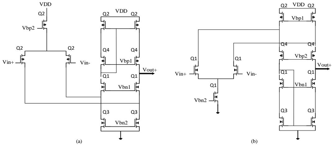
Figure 8. Gain-booster auxiliary amplifiers (a) PMOS-input stage (b) NMOS-input stage
