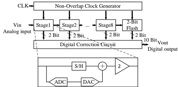
Figure 1. Pipelined ADC architecture
