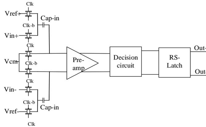
Figure 3. Schematic diagram of clocked comparator
