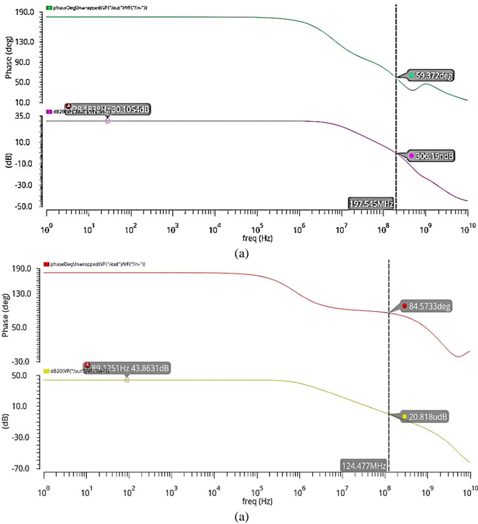
Figure 9. AC responses for gain-booster auxiliary amplifiers: (a) NMOS-input op-amp and (b) PMOS-input op-amp
