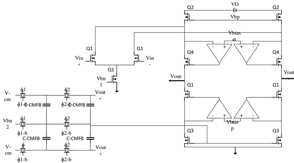
Figure 7. Schematic of gain-boosted amplifier
