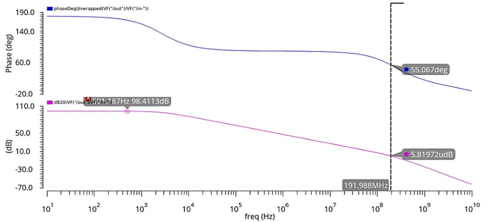
Figure 10. AC Responses for the gain-boostered op-amp
