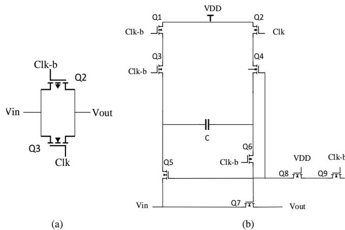
Figure 11. Switches (a) CMOS TG and (b) Bootstrapped switch
