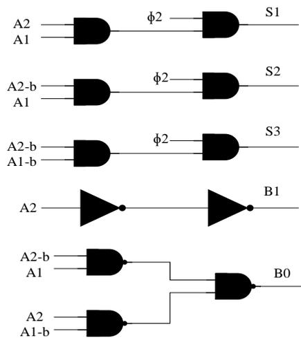
Figure 6. Sub-ADC logic circuit
