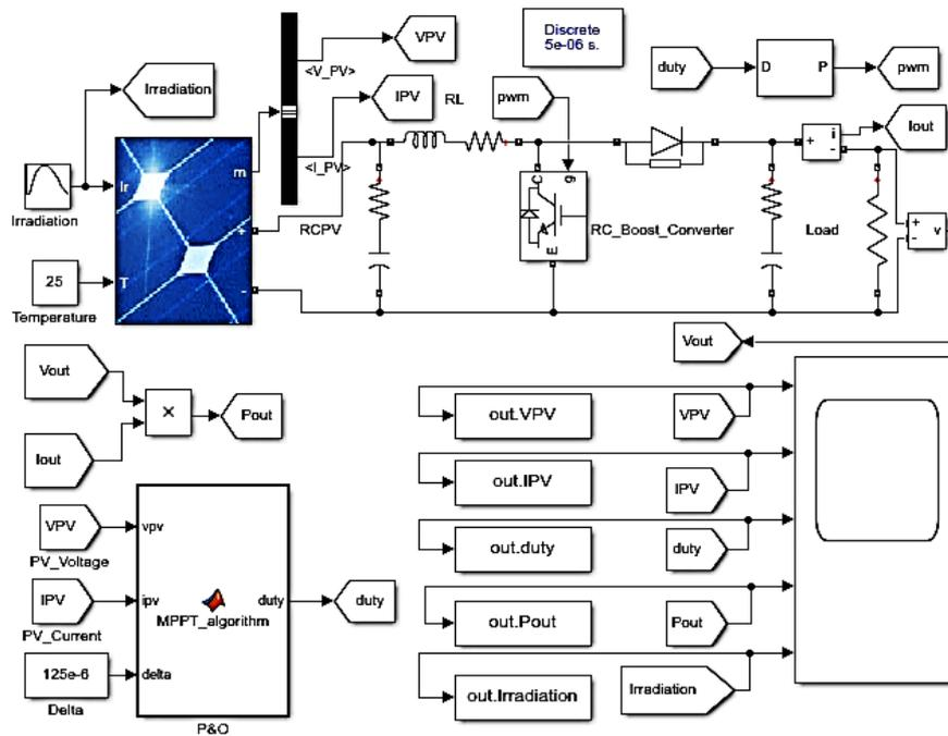
Figure 6. The block diagram of P&O MPPT controller
