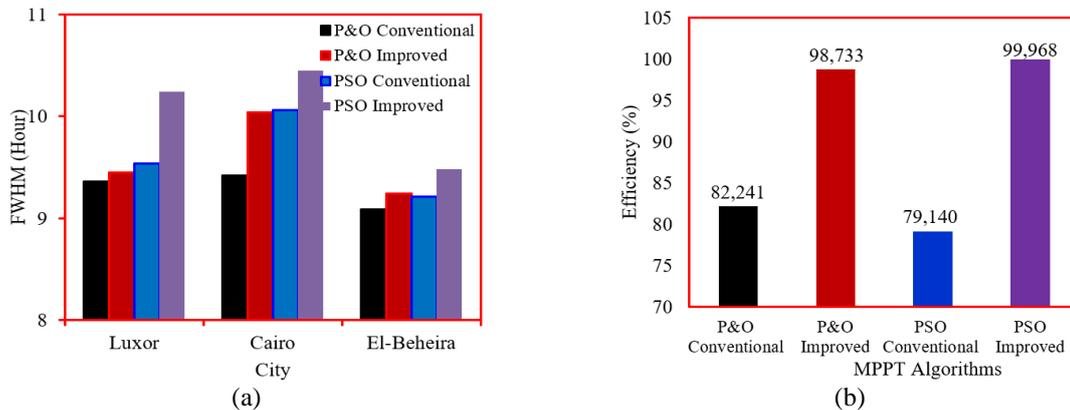
Figure 14. Comparison between the conventional and improved of P&O and PSO (a) FWHM and (b) efficiency
