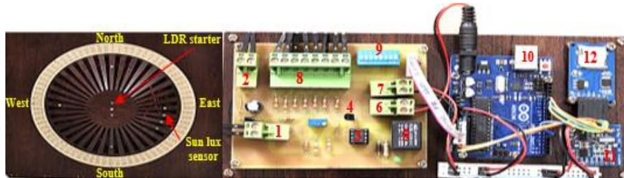
Figure 3. Solar irradiance tracer control system: 1) LDR starter, 2) 9 V from adaptor, 3) operational amplifier, 4) transistor BC547BP, 5) relay 9 V, 6) 9 V to Arduino, 7) 5 V from Arduino, 8) 7 jumpers from LDRs, 9) switch from 7 jumpers from LDRs to analog pins of Arduino, 10) Arduino uno, 11) RTC module, and 12) SD memory card
