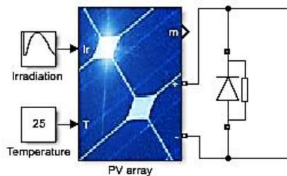
Figure 4. PV array model of the present study
