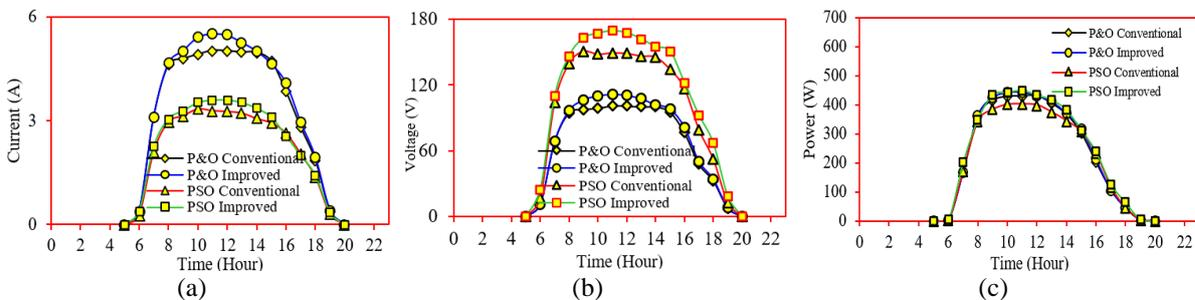
Figure 13. Comparing the obtained simulation results using conventional P&O, conventional PSO, improved P&O, and improved PSO for El-Beheira city in (a) output current, (b) output voltage, and (c) output power
