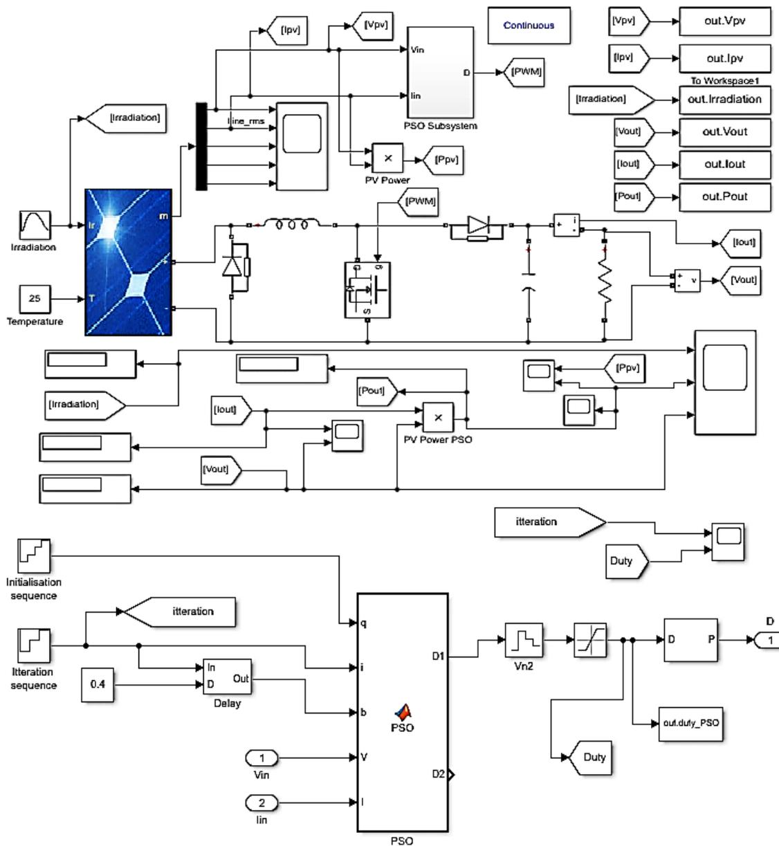
Figure 7. The block diagram of PSO MPPT controller and the subsystem of PSO algorithm
