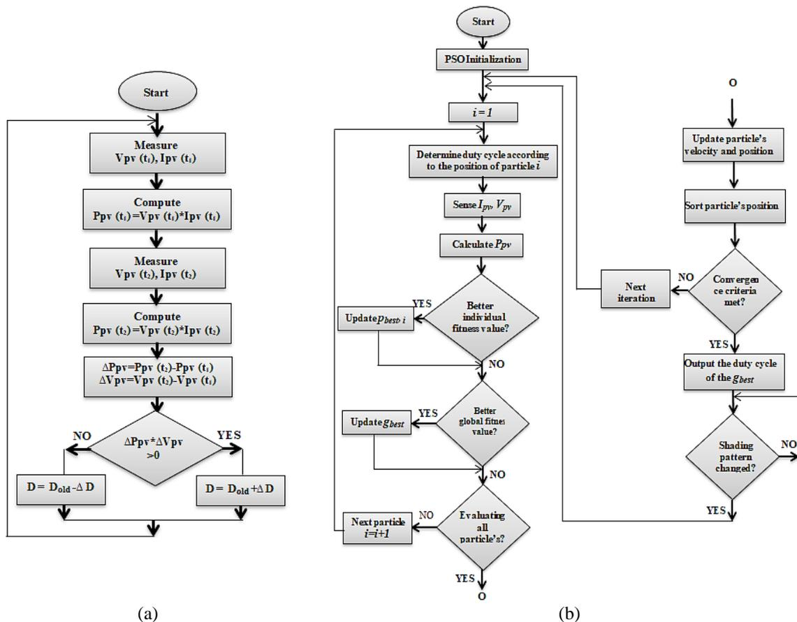
Figure 8. The improved flowchart (a) P&O and (b) PSO
