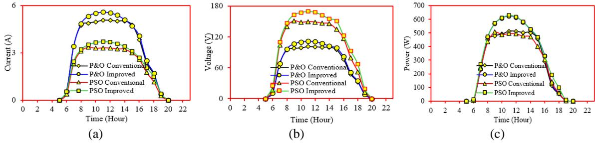
Figure 11. Comparing the obtained simulation results using conventional P&O, conventional PSO, improved P&O, and improved PSO for Luxor city in (a) output current, (b) output voltage, and (c) output power
