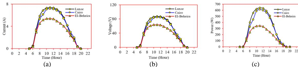
Figure 10. Comparing the simulation results of PV array for the three studied regions in (a) output current, (b) output voltage, and (c) output power
