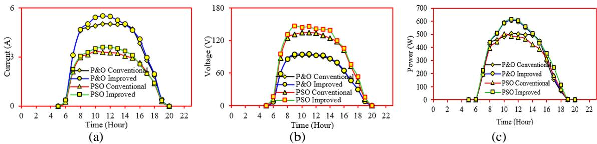
Figure 12. Comparing the obtained simulation results using conventional P&O, conventional PSO, improved P&O, and improved PSO for Cairo city in (a) output current, (b) output voltage, and (c) output power
