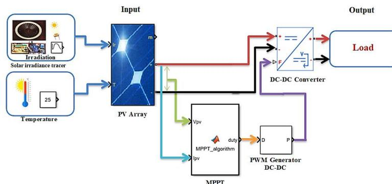
Figure 2. The block diagram of the proposed system
