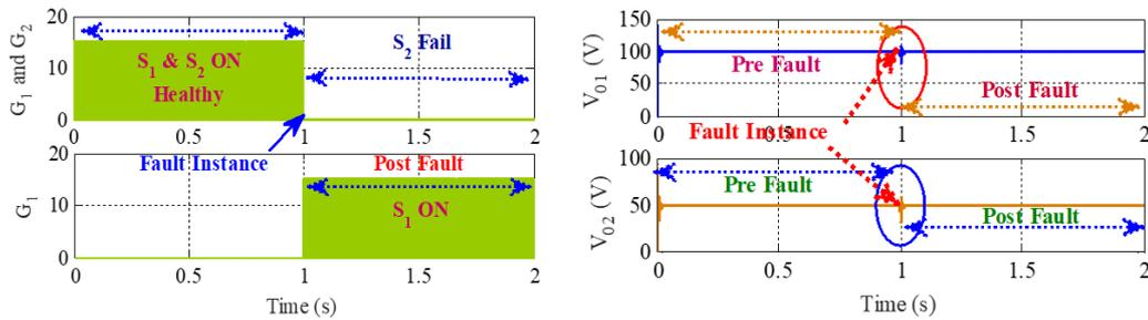
Figure 8. Simulation gate pulses for switches and output voltage during  $S_2$  failure case
