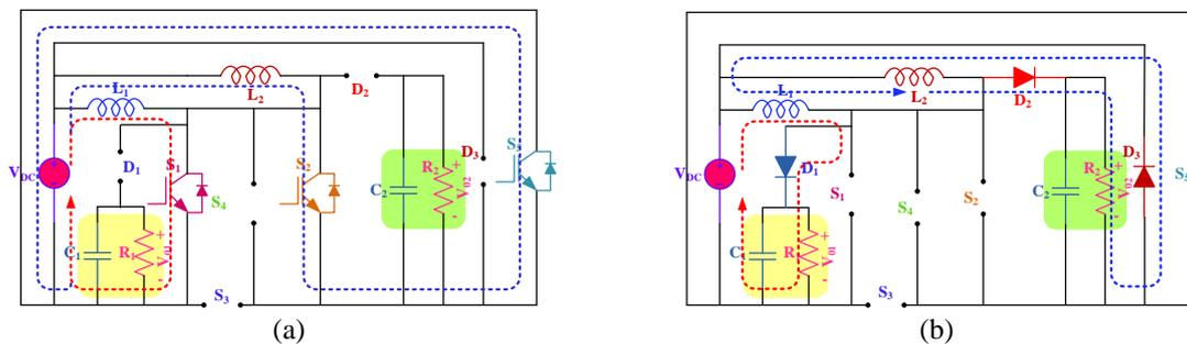
Figure 2. Switching states: (a) mode 1 and (b) mode 2
