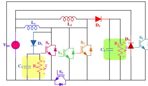
Figure 1. Schematic of proposed fault-tolerant SIDO configuration
