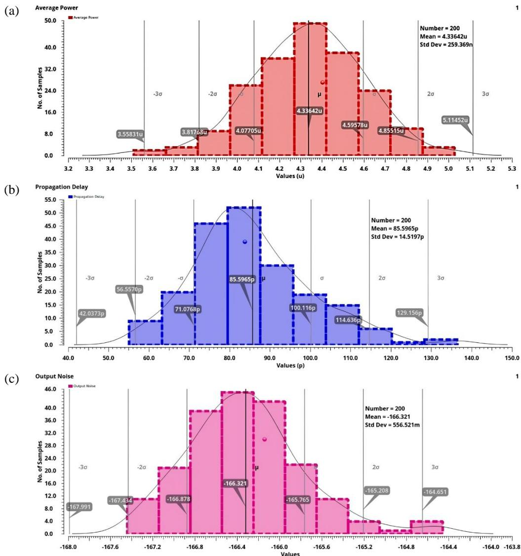
Figure 6. Monte carlo analysis for the proposed LVF D-Latch of (a) power, (b) propagation delay, and (c) noise
