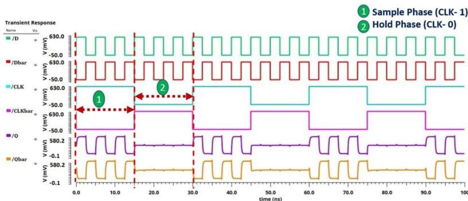
Figure 5. Transient response of the proposed LVF D-Latch
