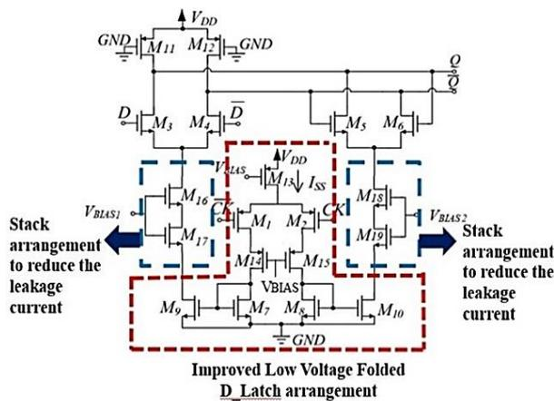
Figure 3. Proposed LVF MCML D-Latch
