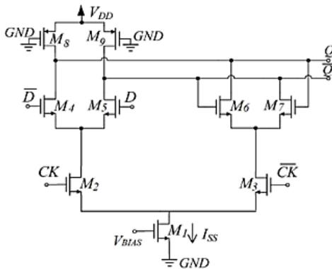
Figure 1. Conventional MCML D-Latch [28]
