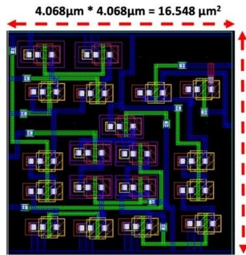
Figure 4. Layout design of proposed D-Latch
