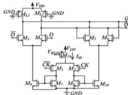
Figure 2. Existing folded MCML D-Latch [29]
