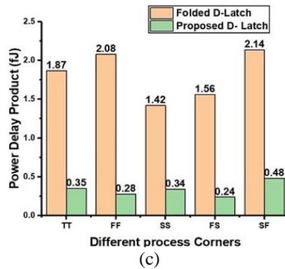
Figure 10. Performance comparison of D-Latch with different process corners vs (a) power, (b) propagation delay, and (c) power delay product
