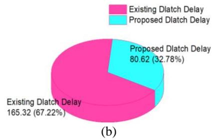
Figure 9. Performance improvement in percentage of (a) power and (b) propagation delay
