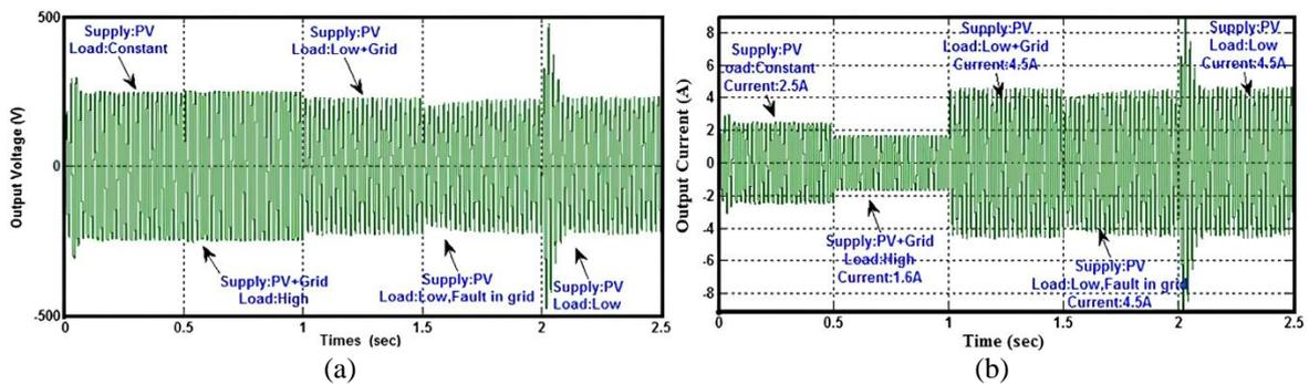
Figure 8. When a load is changing, (a) the output voltage and (b) the current through a GA PID controller
