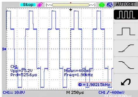
Figure 11. Bidirectional inverter's output voltage
