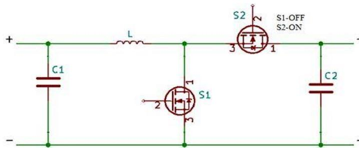
Figure 4. BDC circuit diagram at boost mode
