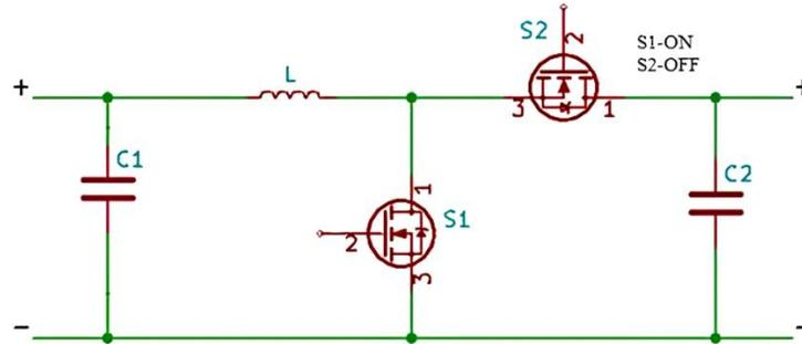
Figure 3. BDC circuit diagram at buck mode
