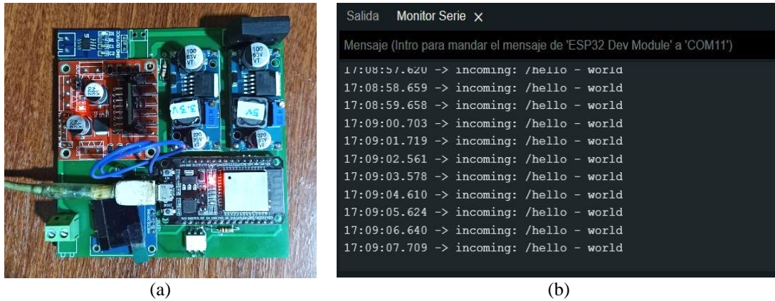
Figure 5. Board: (a) uploading the code and (b) performing link testing via WIFI
