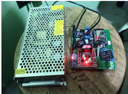
Figure 8. Implementation and installation of the components on the board designed for the management and monitoring of lithium-ion battery recharging
