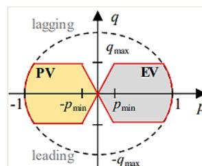
Figure 2. Permissible range of reactive power for a power generation system:  $3.68 \text{ kVA} < \sum S_{E_{max}} \leq 13.8$  [23]
