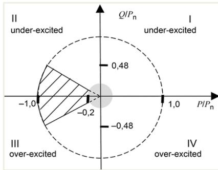
Figure 3. Boundaries for reactive power in a power generation system:  $\sum S_{E_{max}} > 13.8$  kVA [23]
