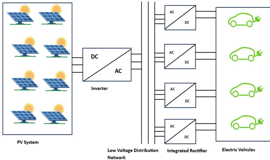
Figure 6. Diagram of the proposed EV recharging station
