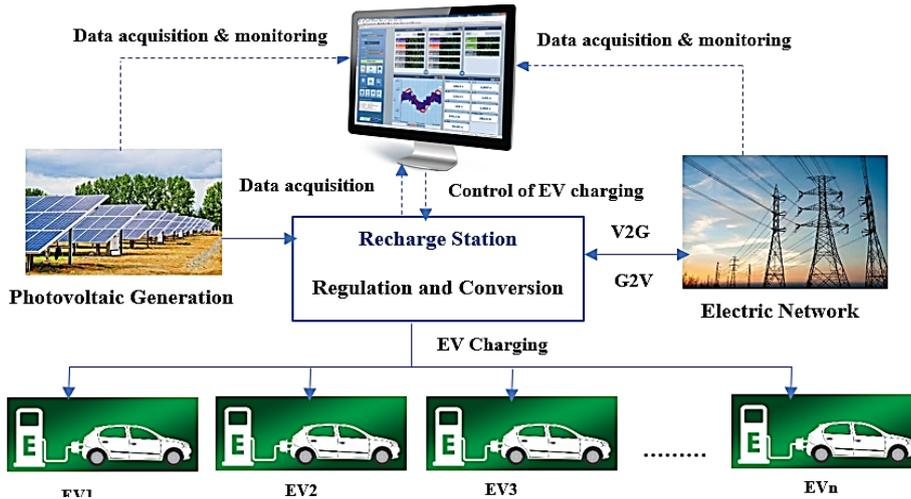
Figure 7. Schematic diagram of recharging unit for EVs
