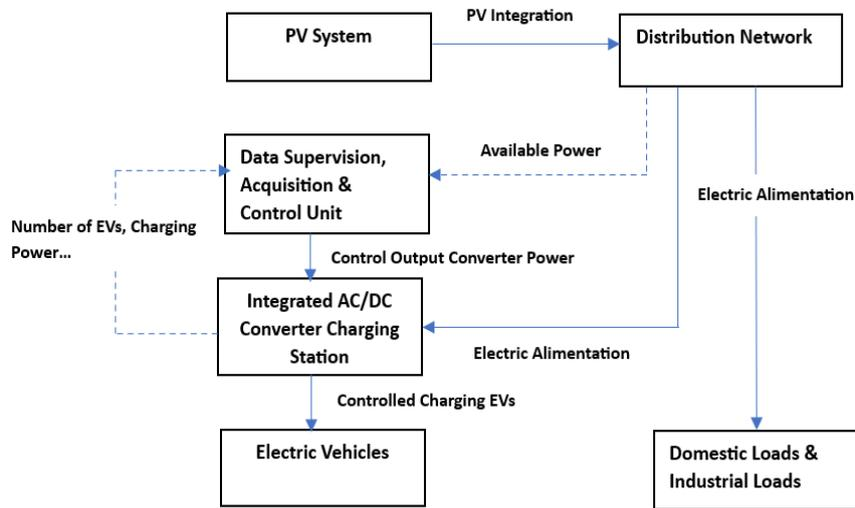
Figure 8. Block diagram of proposed charging method
