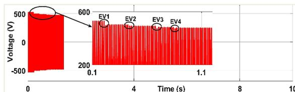
Figure 9. Voltage drops after EVs integration
