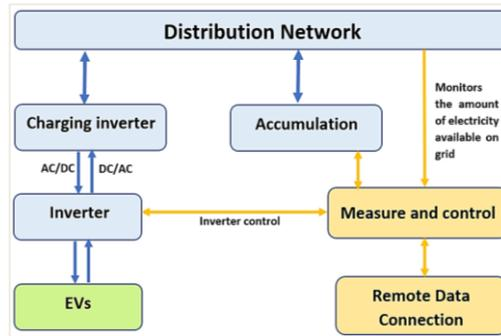
Figure 1. Architecture of EVs charging station [4]
