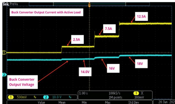
Figure 25. Output voltage and output current waveforms
