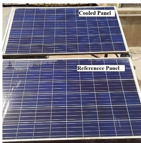
Figure 3. Experimental PV panel setup
