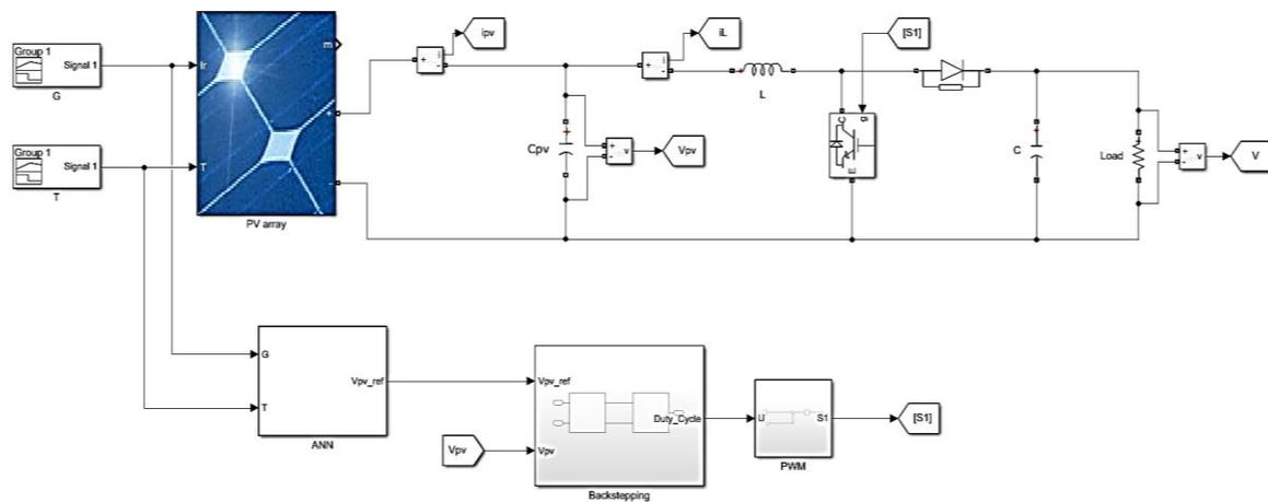
Figure 6. Simulation model of proposed system
