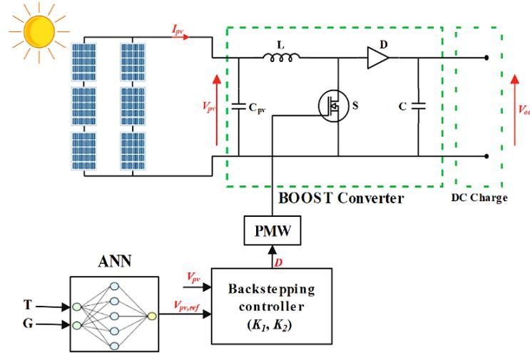
Figure 3. Control design of the system
