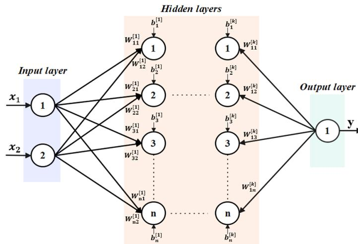
Figure 4. Architecture of the feedforward
