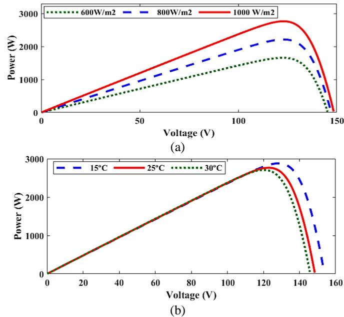
Figure 1. PV characteristic of the PV array (a) at variable solar irradiance and (b) at variable temperature
