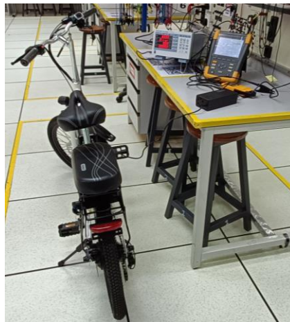
Figure 2. Set up wire-connected charging tests
