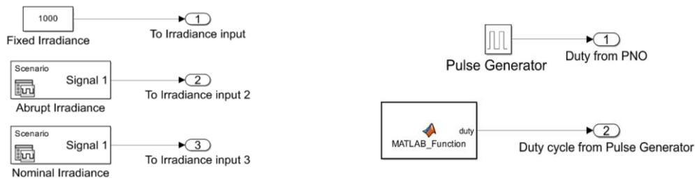
Figure 3. Simulation blocks of irradiance settings Figure 4. Simulation blocks of control switching technique
