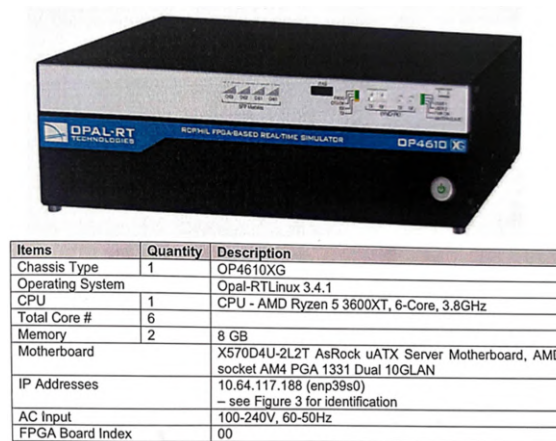
Figure 6. OP4610XG real time simulator and features of target computer
