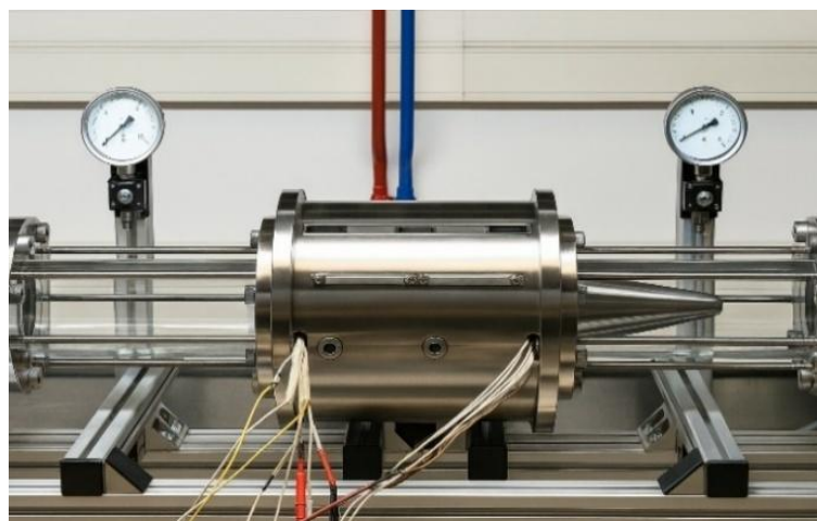
Figure 8. Prototype of the counter-rotating micro-hydro turbine with its two PM-generators [32]
