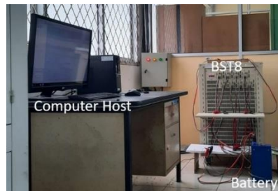
Figure 1. Physical representation of the experimental platform for testing Lithium-ion batteries
