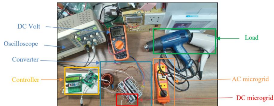
Figure 11. Photograph of the experimental converter in the laboratory, experimental measurement of the operating parameters of the proposed AC/DC converter
