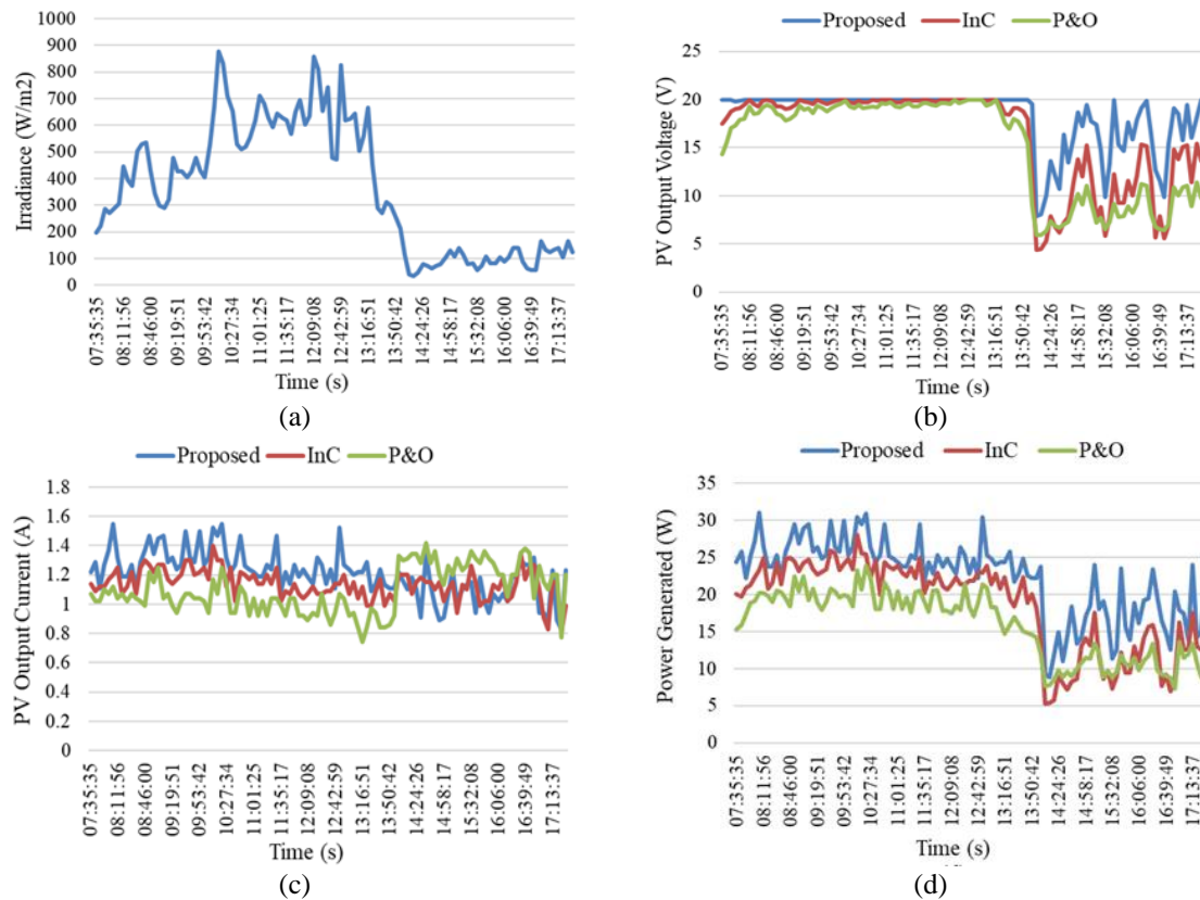
Figure 9. The system test results on the third day: (a) irradiance, (b) PV output voltage, (c) PV output current, and (d) power generated
