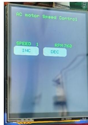
Figure 4. Display of speed in RPM at level-1
