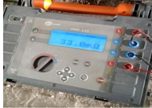
Figure 7. MMR-620 continuity test value
