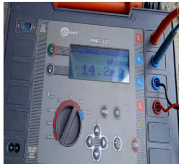
Figure 9. MMR-620 continuity test for random MS solid round conductor
