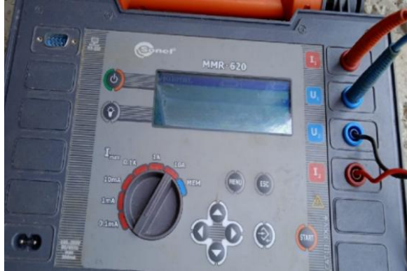
Figure 6. MMR-620 continuity test device in off position
