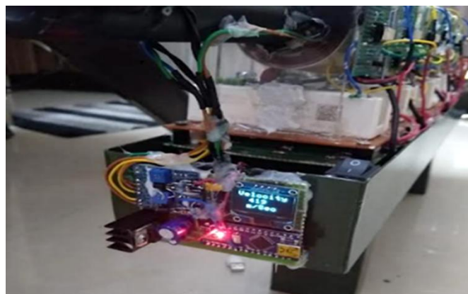
Figure 16. Bullet velocity measured in a 6-stage coil gun
