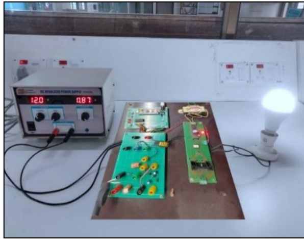
Figure 8. Hardware setup of NI-Cuk with Vfc
