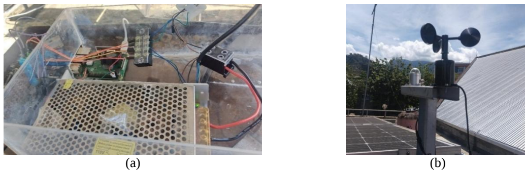
Figure 3. Forecasting system: (a) the Raspberry Pi-based monitoring and power supply unit, and (b) the outdoor solar irradiance and wind speed sensors
