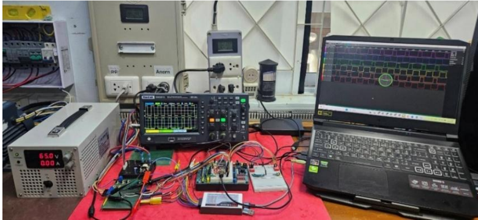
Figure 6. Experimental hardware platform for the proposed capacitor-less PSC motor drive
