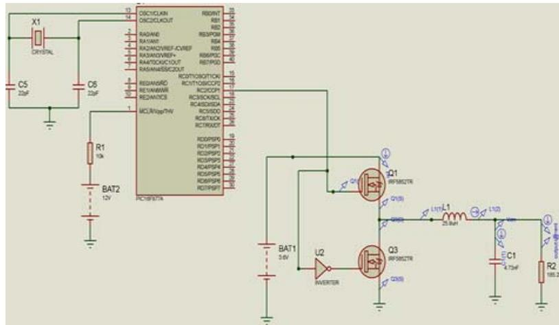
Figure 3. The simulation model of half-bridge Class D parallel resonant inverter
