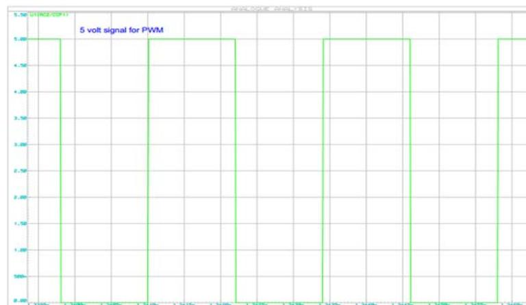
Figure 4. Simulation waveform of PWM
