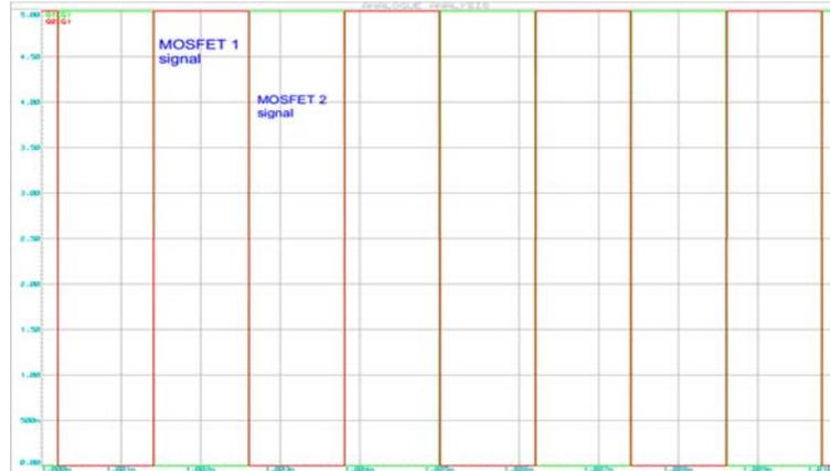
Figure 5. Simulation waveform for MOSFET gate signal
