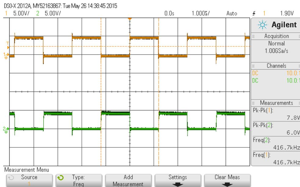
Figure 8. Gate signal for MOSFET
