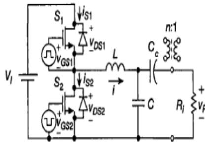
Figure 2. The standard model of half-bridge Class D parallel resonant inverter[23]
