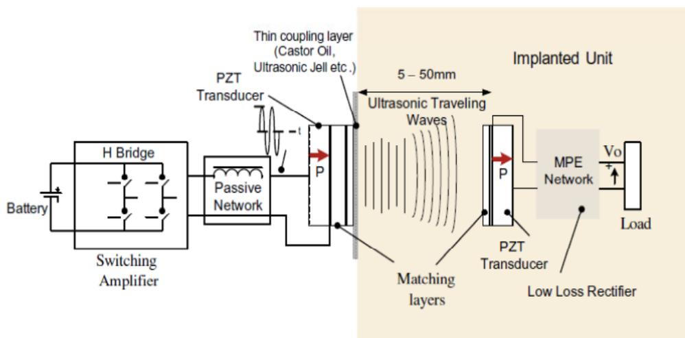
Figure 1. Acoustics Energy Transfer System [4]
