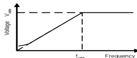
Fig. 6 Voltage versus frequency under the constant V/Hz principle
