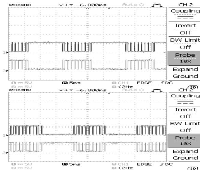
Fig.17. Phase R pulses from DSP Controller.
