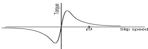
Fig.7 Torque versus slip speed of an induction motor with constant stator flux
