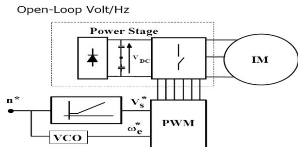
Fig 5 Open –Loop Volt/Hz
