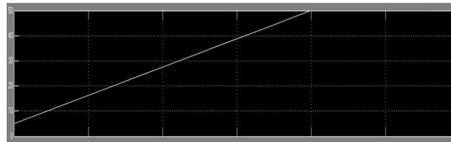
Fig 12. V/f profile (frequency from 5-50Hz)
