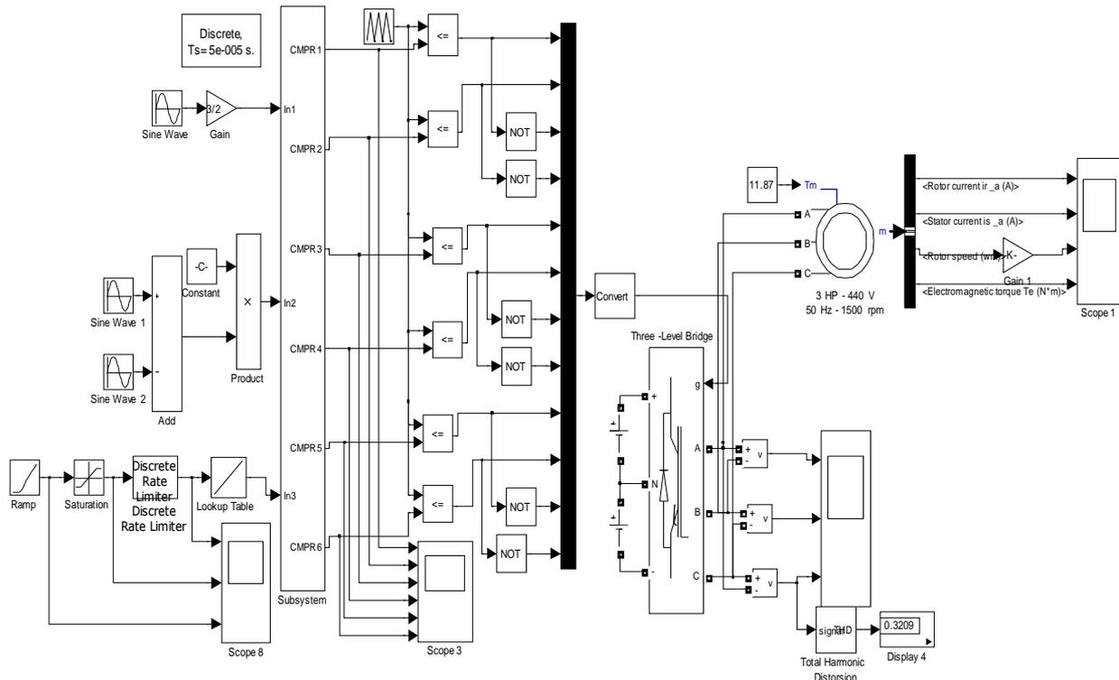
Fig.9. Simulink block of Scalar Control
