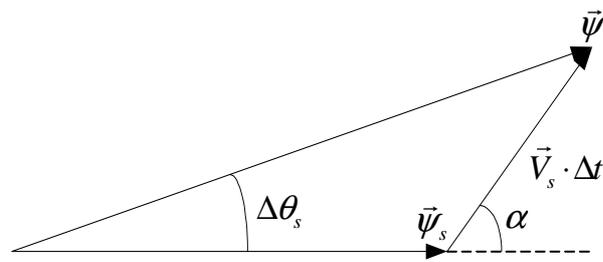
Figure 1. The move of stator flux vector
