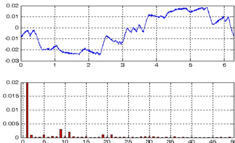
Figure 32 FFT of a-phase stator current @ load
