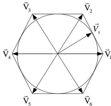
Figure 14 The amplitude of applied voltage vector
