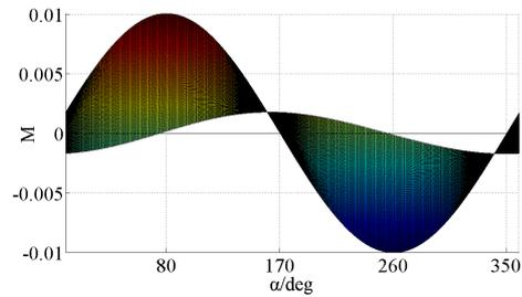
Figure 5 The change of torque @  $\delta=10^\circ$
