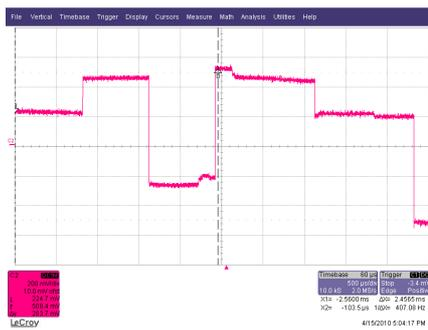
Figure 24 The a-phase stator voltage (40V/div) @ no-load
