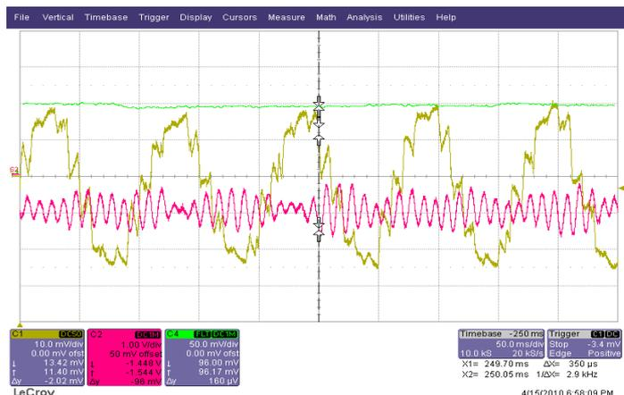
Figure 31 The a-phase stator current (yellow, 20A/div), motor speed (green, 50rpm/div) and load torque (red, 10Nm/div) @ load
