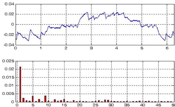
Figure 26 FFT of a-phase stator current @ load
