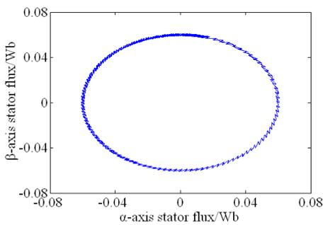
Figure 19 Stator flux circle
