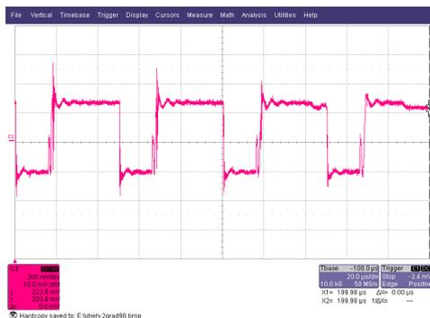
Figure 30 The a-phase stator voltage (40V/div) @ no-load
