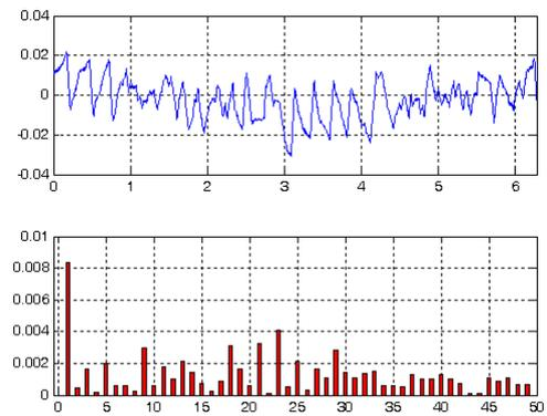
Figure 29 FFT of a-phase stator current @ empty load
