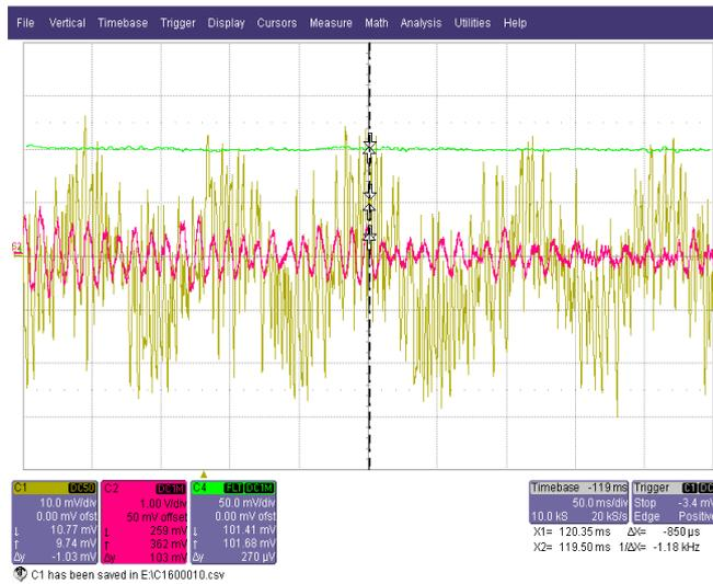
Figure 28 The a-phase stator current (yellow, 5A/div), motor speed (green, 50rpm/div) and load torque (red, 10Nm/div) @ no-load
