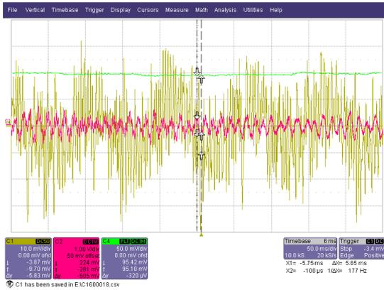
Figure 22 The a-phase stator current (yellow wave, 5A/div), motor speed (green wave, 50rpm/div) and load torque (red wave, 10Nm/div) @ no-load
