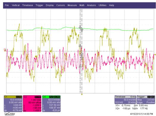
Figure 25 The a-phase stator current (yellow, 20A/div), motor speed (green, 50rpm/div) and load torque (red, 10Nm/div) @ load
