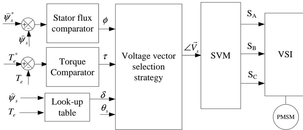
Figure 16 The interior PMSM DTC drive using voltage vector selection strategy
