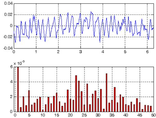
Figure 23 FFT of a-phase stator current @ empty load
