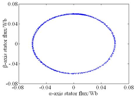
Figure 17 Stator flux circle
