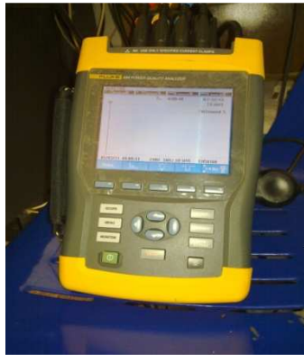
Figure 1 Power Quality Analyzer
