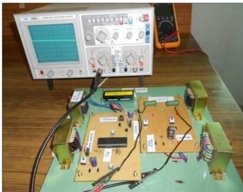
Figure 8(b). Output Measured with Oscilloscope (Scale: y-axis: 1 div and 10Volts/div)
