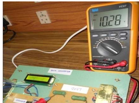
Figure 8(a) Output Voltage Measured using Multimeter
