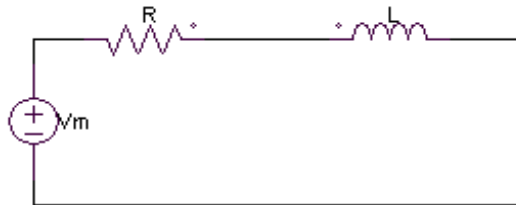
Figure 1. Electrical Model of One Phase of SRM
