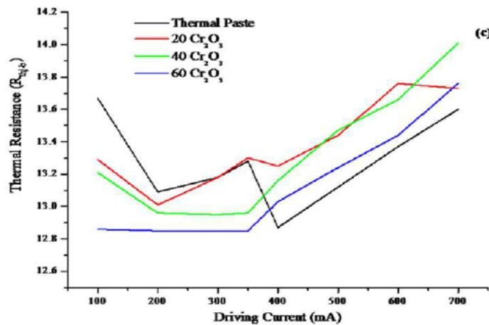
Figure 6. Change in (a) total thermal resistance ( $R_{th,tot}$ ), (b) board to heat sink thermal resistance ( $R_{th,b-hs}$ ) and (c) junction to board thermal resistance for various  $\text{Cr}_2\text{O}_3$  concentrations at different driving current.
