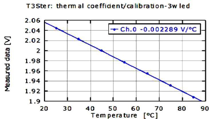
Figure 2. K factor calibration curve.
