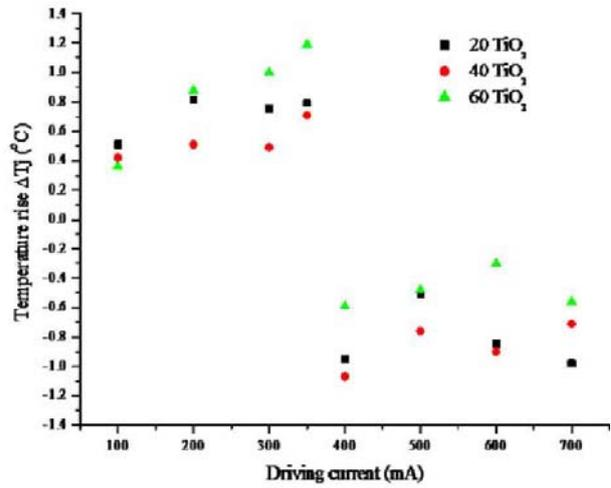
Figure 5. Variation in junction temperature rise for different in TIM with respect to driving current
