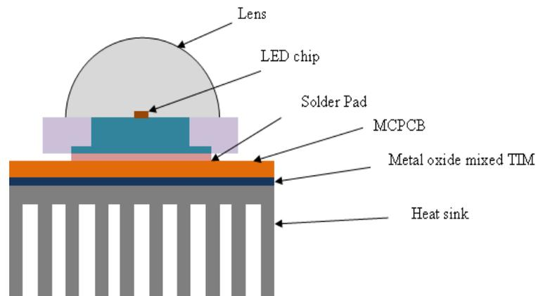
Figure 1. Schematic diagram of device under test showing metal oxide filled TIM sandwiched between LED package and heat sink
