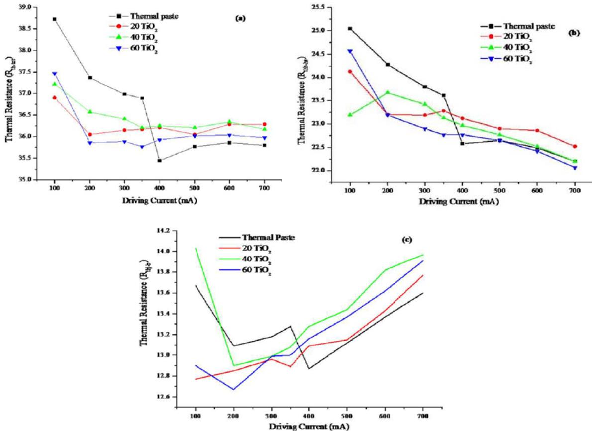
Figure 7. Change in (a) total thermal resistance ( $R_{th-tot}$ ), (b) board to heat sink thermal resistance ( $R_{th-b-hs}$ ) and (c) junction to board thermal resistance for various  $TiO_2$  concentrations at different driving current
