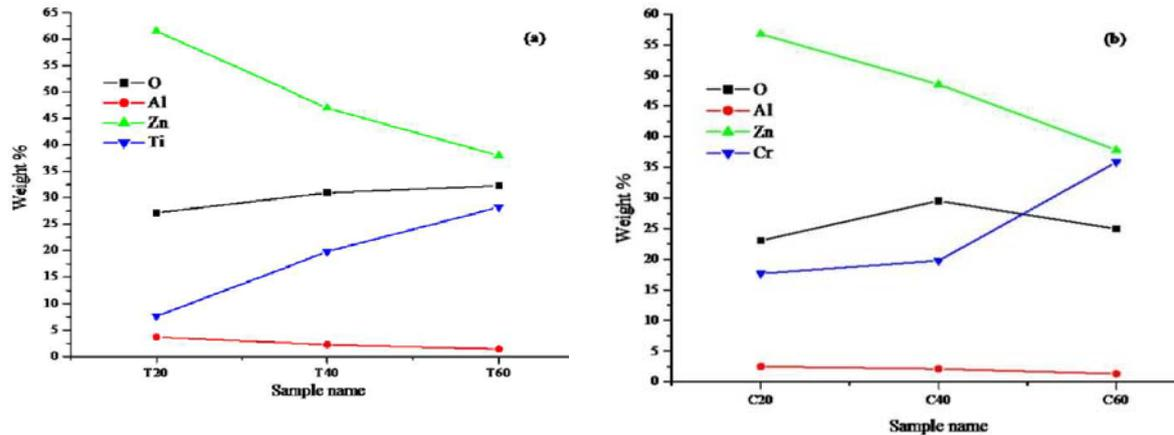
Figure 8. Elemental weight percentage available in (a) TiO<sub>2</sub> mixed TIM for different TiO<sub>2</sub> mixed ratio and (b) Cr<sub>2</sub>O<sub>3</sub> mixed TIM for different TiO<sub>2</sub> mixed ratio.
