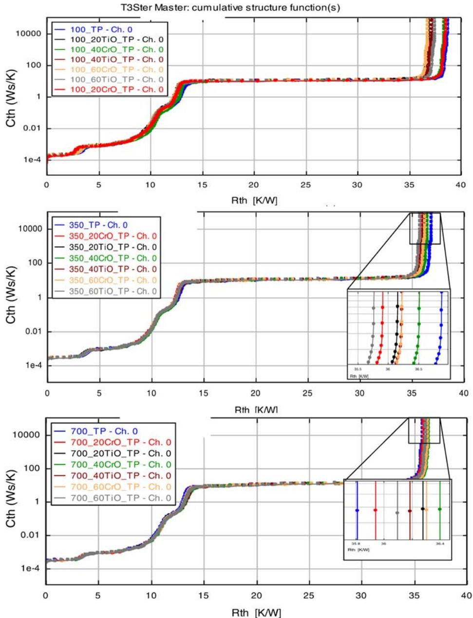
Figure 3 Cumulative Structure Function of 3W green LED for different metal oxide ( $\text{TiO}_2$  and  $\text{Cr}_2\text{O}_3$ ) mixed TIM measured at (a) 100 mA driving current, (b) 350 mA driving current and (c) 700 mA driving current
