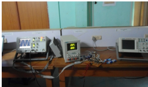
Figure 4. Experimental setup of proposed inverter
