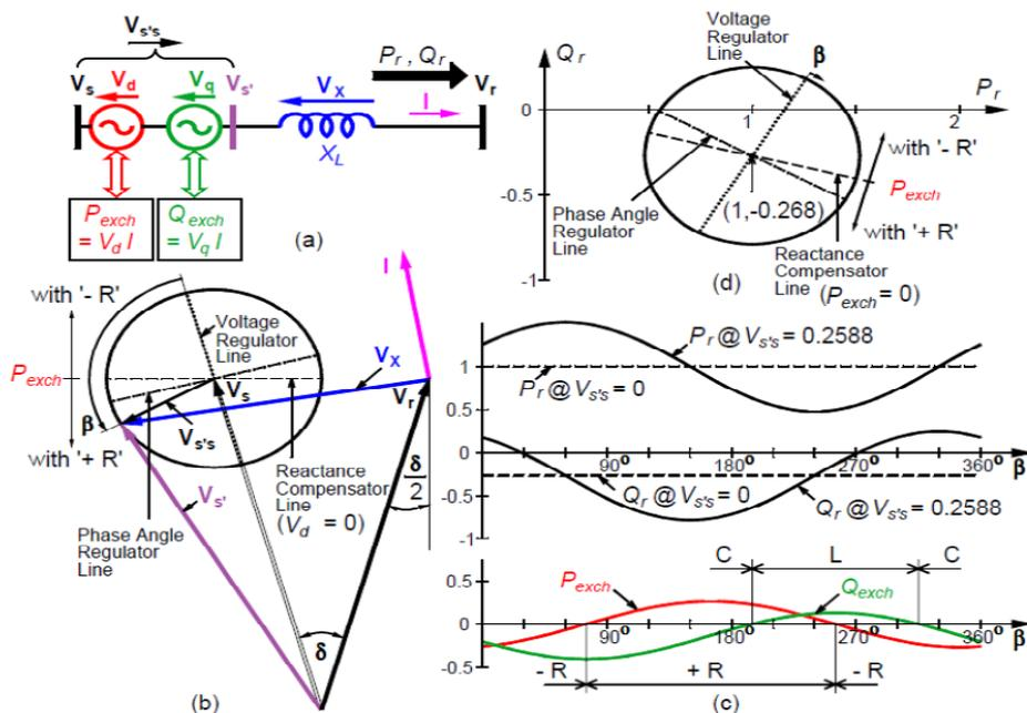
Figure 4. Effect of a series-connected voltage source on power flow in a transmission Line. (a) Power transmission system with a series-connected compensating voltage,  $V_s's$ , (b) phasor diagram, (c) variation of the receiving-end real and reactive power ( $P_r$  and  $Q_r$ ) and the exchanged compensating real and reactive power as a function of the angular rotation of the compensating voltage phasor, and (d) receiving-end  $Q_r$  vs.  $P_r$ .
