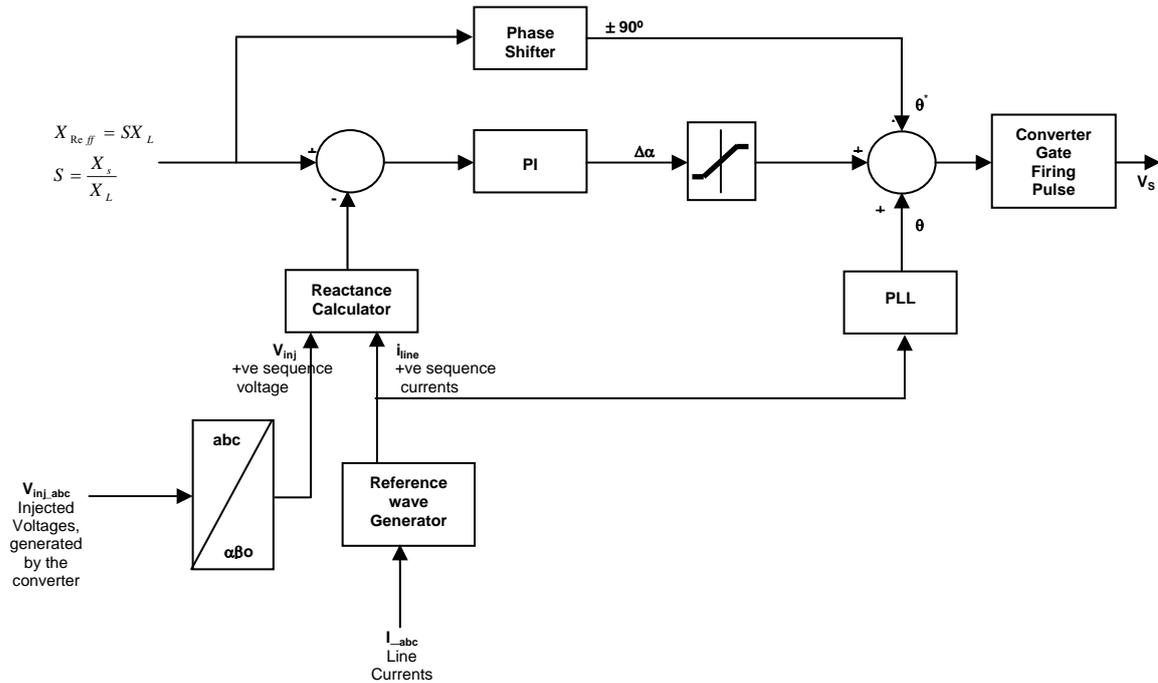
Figure 9. Basic Control Block for SSSC
