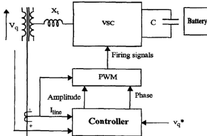
Figure 8. Basic Control block of SSSC
