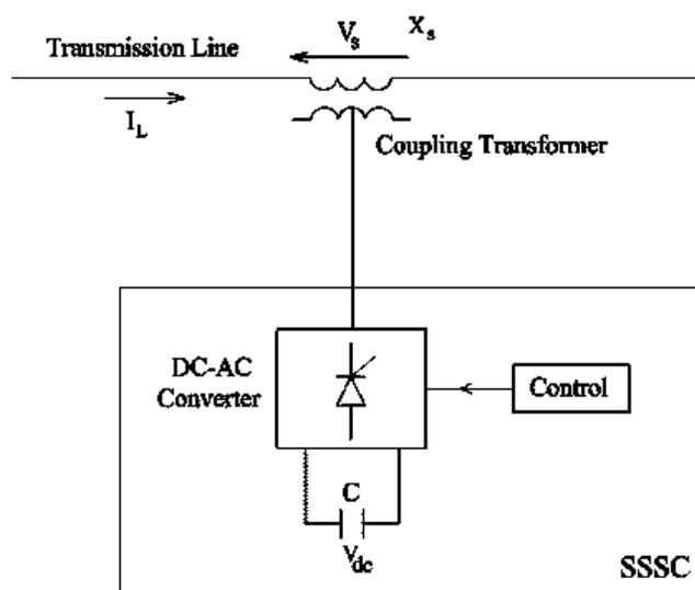
Figure 1. Basic Building block of SSSC
