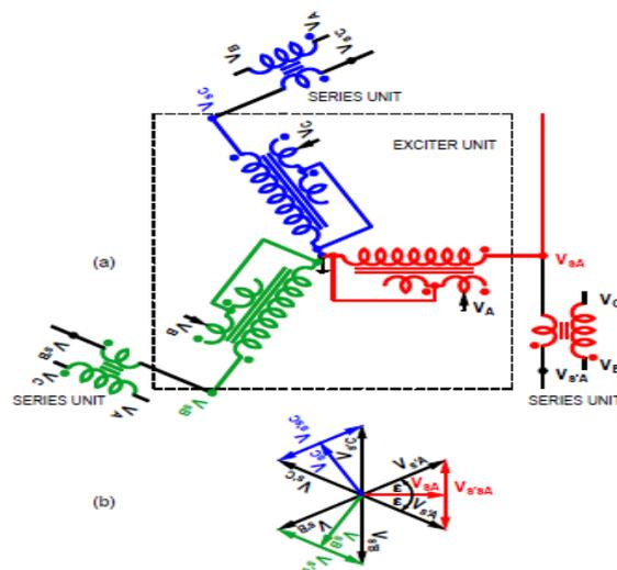
Figure 3. (a) Phase angle regulator circuit (b) phasor diagram
