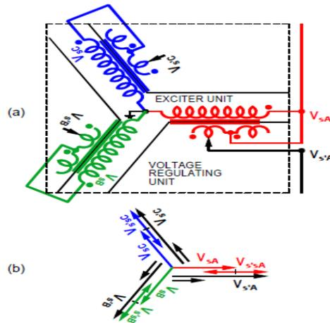
Figure 2. (a) Voltage regulator circuit (b) phasor diagram
