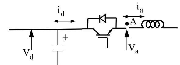
Figure 7. Single valve operation
