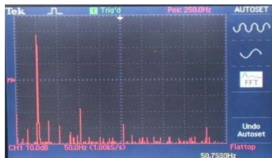
Figure 15. Harmonic spectrum of output voltage
