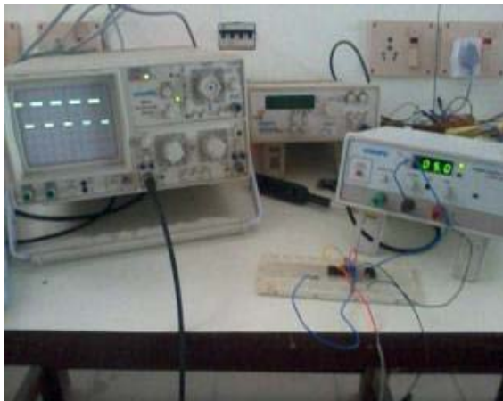
Figure 7. Output obtained from PIC circuit for firing MDIBC
