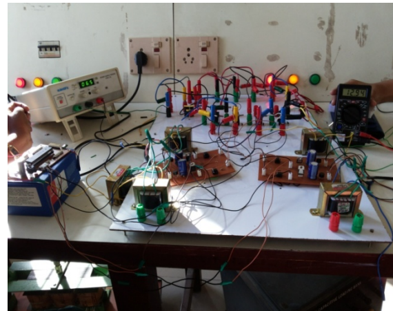
Figure 8. A Prototype of Multi device Interleaved Boost converter with optocouplers and PIC circuit
