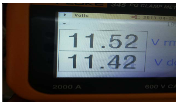
Figure 9. Output voltage of MDIBC measured using PQ analyzer
