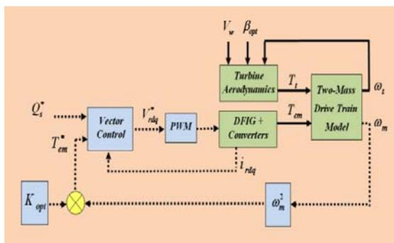
Figure 9. Block diagram of OT control MPPT method
