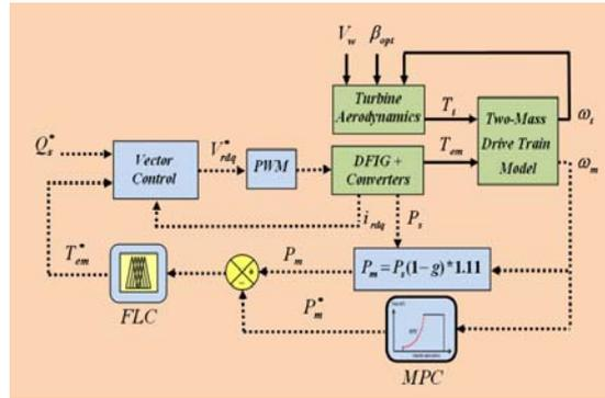
Figure 8. Block diagram of MPCS-MPPT control system
