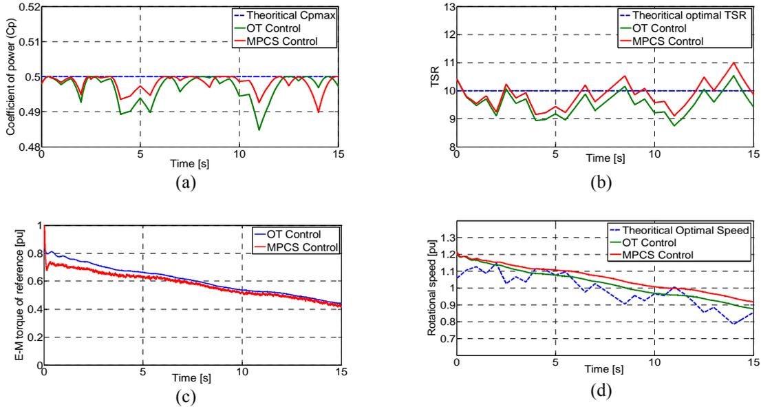
Figure 12. Dynamic response comparison between OT and MPCS control techniques
