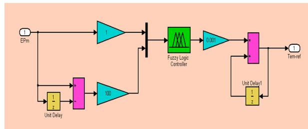
Figure 6. FLC structure of the mechanical power
