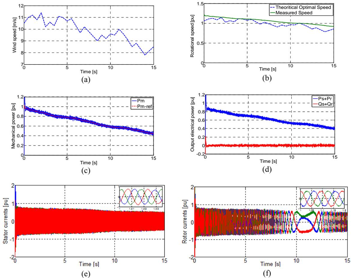
Figure 11. Dynamic responses of the fuzzy-MPCS algorithm in the variable speed mode
