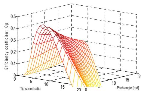
Figure 10. Power coefficient curve versus TSR and pitch angle
