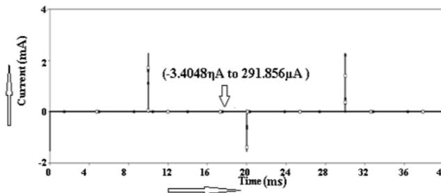
Figure 12(a). Leakage current in between PV panel to ground
