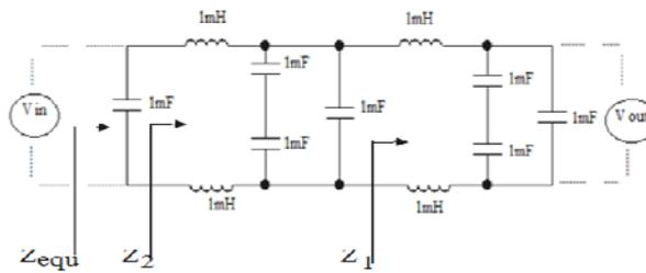
Figure 4. EMC Filter with 10V, 50Hz input [15]
