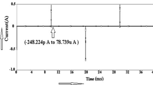
Figure 12(e). Leakage current in between AC decoupling switches
