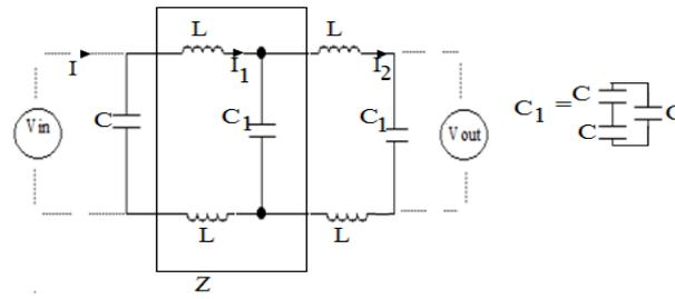
Figure 5. Current directions for finding transfer function
