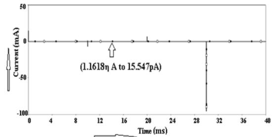
Figure 13(c). Leakage current of an inverter after using 100 ohm resistance
