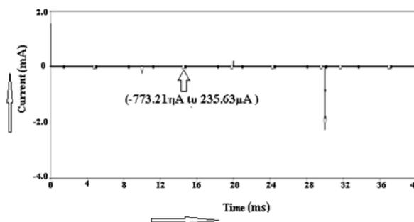
Figure 13(a). Leakage current in between PV panel to Ground
