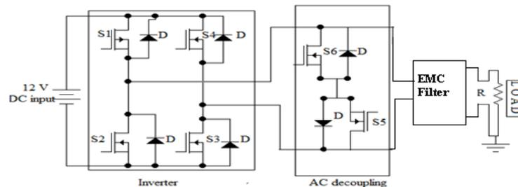
Figure 10. AC-decoupling based transformers-less inverter topology [18]
