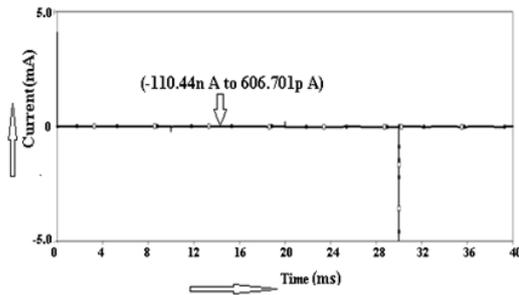
Figure 13(b). Leakage current shoes in the inverter
