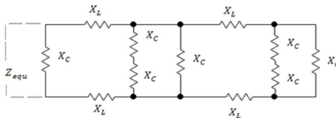
Figure 6. Equivalent impedance of EMC Filter
