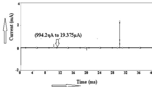
Figure 13(d). Leakage current in between switch S1 and S2
