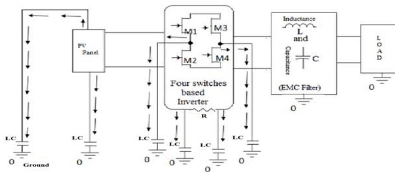
Figure 11. Approach topology where leakage paths are shown
