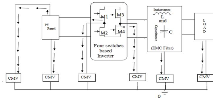
Figure 8. Different leakage current paths
