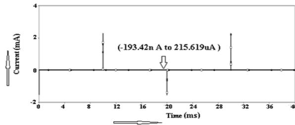
Figure 12(d). Leakage current in between switch S1 and S2
