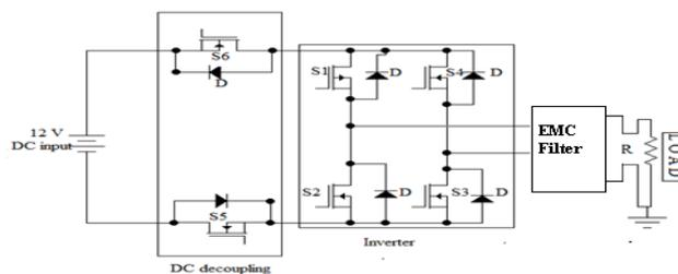
Figure 9. DC-decoupling based transformer-less inverter topology [17]
