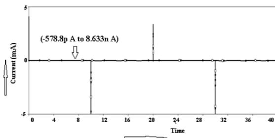
Figure 12(b). Leakage current of an inverter
