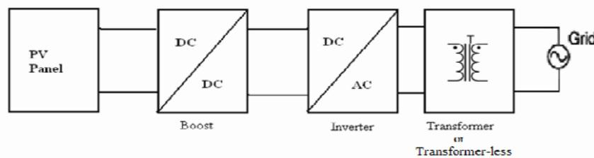
Figure 2. The overall system either transformer-based or transformer-less
