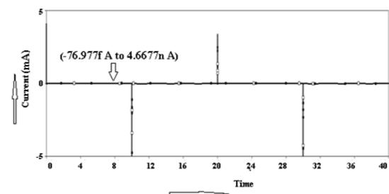
Figure 12(c). Leakage current of an inverter after using tiny resistance
