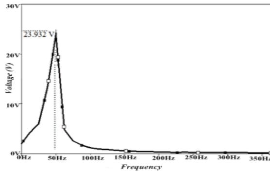
Figure 7. Plot of EMC Filter for 5V input with 50Hz frequency
