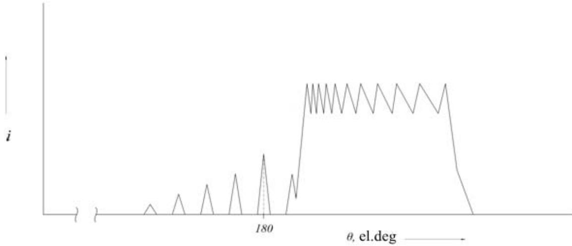
Figure 3. Sensorless controlled SRM phase current
