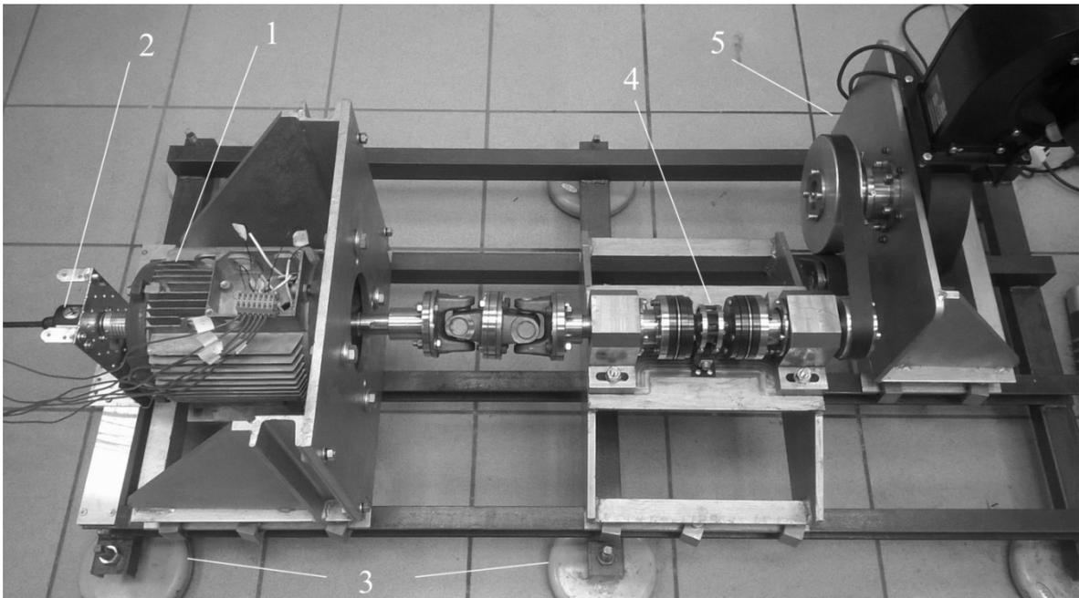
Figure 2. Experimental assembly for noise level measurement
