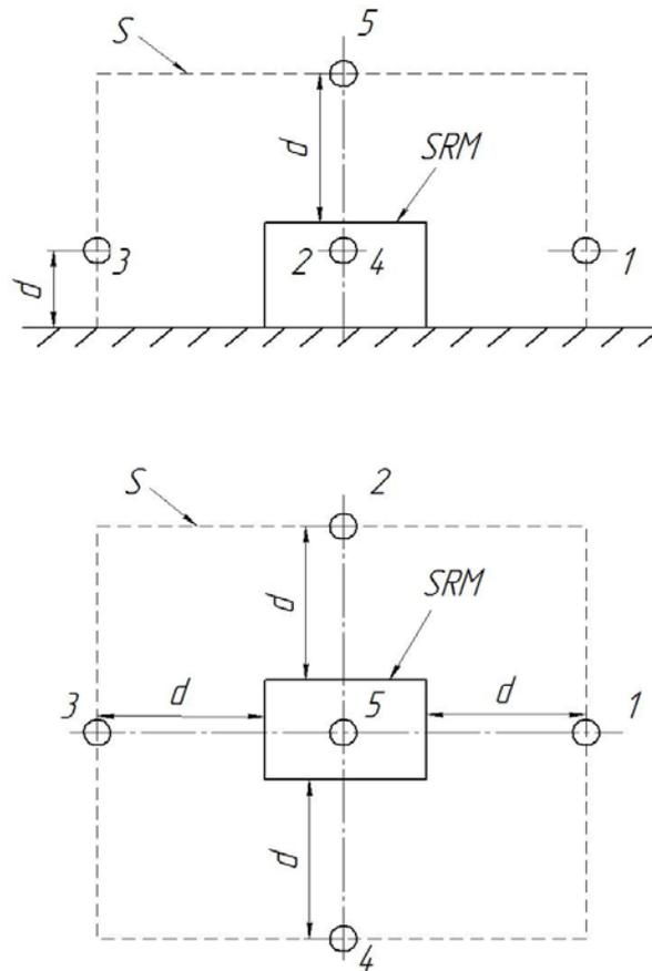
Figure 4. Location of measuring points on the measuring surface
