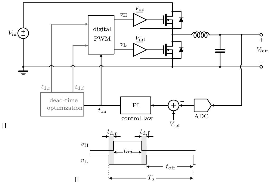
Figure 1. Synchronous buck converter (a) block diagram; and (b) PWM signals with dead time.
