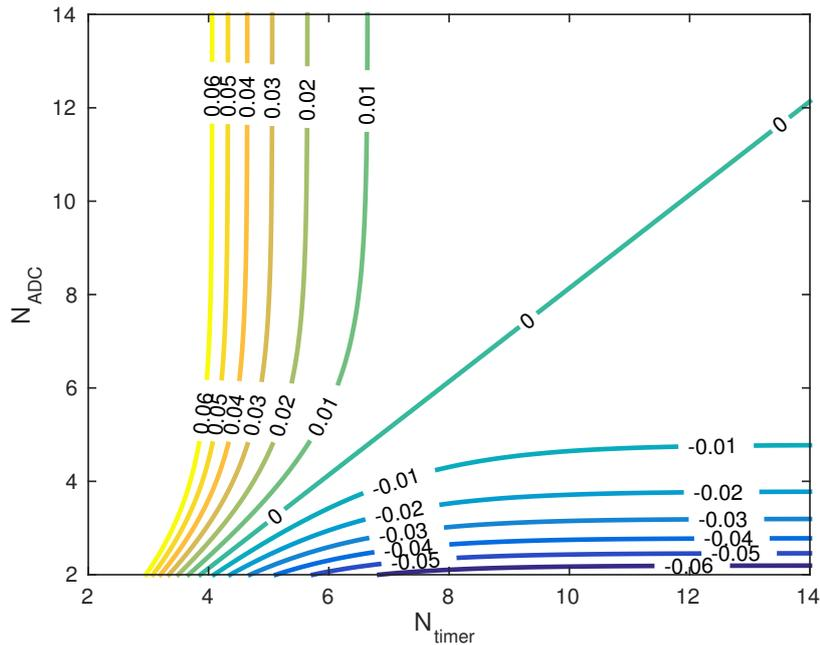
Figure 3. Contour plot of  $\varphi$  for  $V_{ref}/V_{in} = 0.275V$  in terms of number of bits for the timer ( $N_{timer}$ ) and ADC ( $N_{ADC}$ ).
