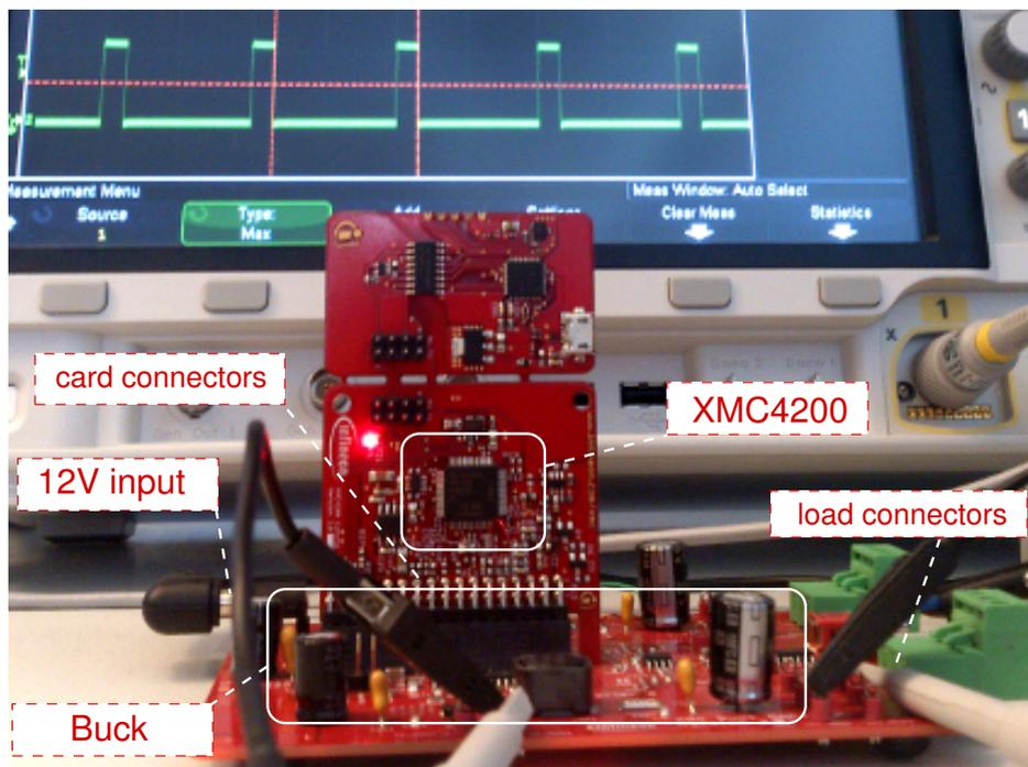
Figure 6. Buck converter and XMC prototype boards.
