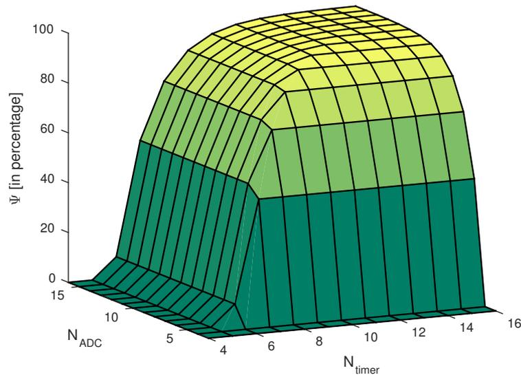
Figure 5. Dependency of the efficiency improvement factor  $\Psi$  with ADC and timer resolutions for  $t_{d,ini} = 400$  ns,  $V_{in} = 12$  V,  $V_D = 0.8$  V,  $V_{ref} = 3.3$  V and  $T_s = 1/320$  kHz.
