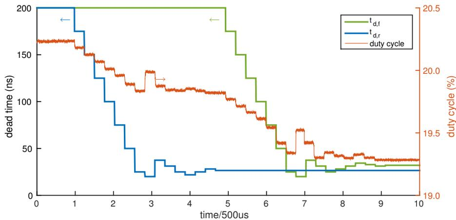
Figure 7. The results of the dead time optimization algorithm, running at slow speed.
