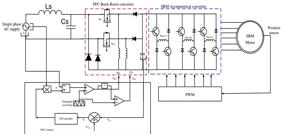
Figure 8. Control Scheme for PWM rectifier fed SRM Drive with PFC Buck-Boost converter
