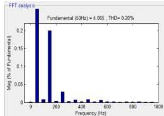
Figure 14. Simulation results THD when the speed is 500 rpm
