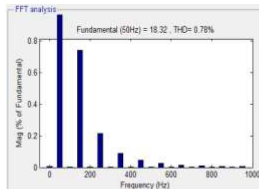
Figure 31. Simulation results THD when there is input variation
