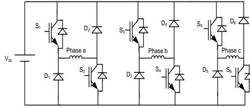
Figure 4. Asymmetrical converter of 6/4 pole SRM Drive
