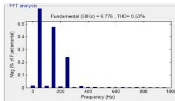
Figure 18. Simulation results THD when the speed is 1000 rpm
