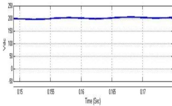
Figure 20. Simulation results of DC link voltage when speed is 1500 rpm
