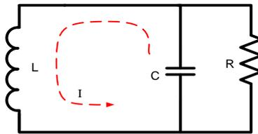
Figure 5(c). Buck-Boost converter switch is OFF
