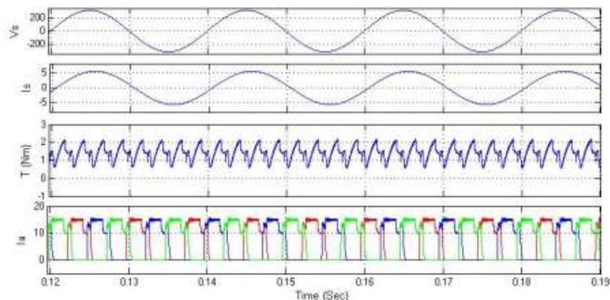
Figure 19. Simulation results of source voltage, source current, torque and armature currents
