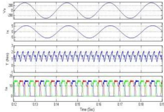
Figure 10. Simulation results of source voltage, source current, torque and armature currents
