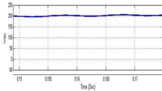
Figure 16. Simulation results of DC link voltage when speed is 1000 rpm
