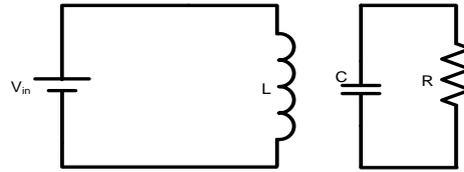
Figure 5(b). Buck-Boost converter switch is ON
