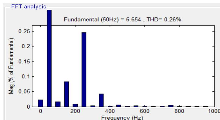
Figure 26. Simulation results THD when the speed is 2000 rpm
