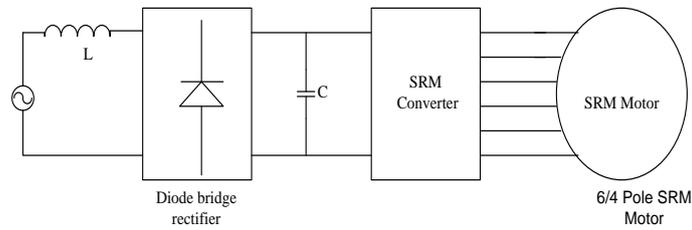
Figure 5. Block diagram of SRM Drive
