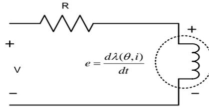
Figure 9. Equivalent circuit of switched reluctance motor
