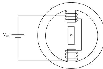
Figure 2. Basic Aligned rotor position
