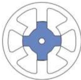
Figure 1. Basic diagram of SRM with 6/4 pole
