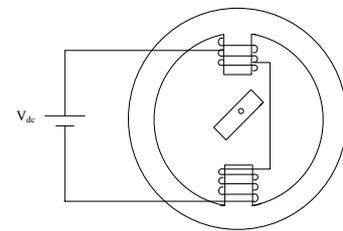
Figure 3. Basic Unaligned rotor position
