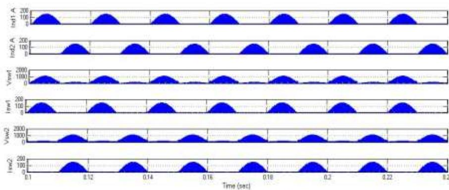
Figure 25. Simulation results of current through inductor 1 and inductor 2, voltage across switches and current through switches 1 and 2
