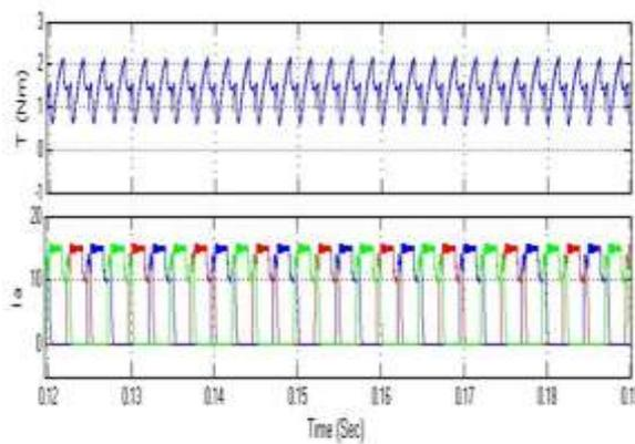
Figure 28. Simulation results of torque and armature currents
