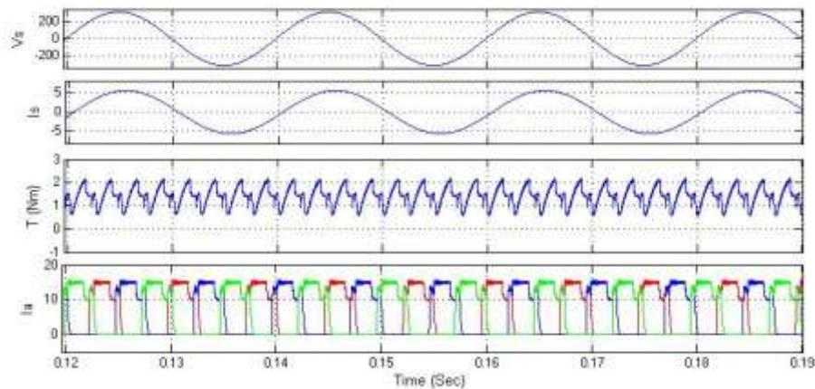
Figure 15. Simulation results of source voltage, source current, torque and armature currents
