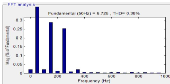
Figure 22. Simulation results THD when the speed is 1500 rpm
