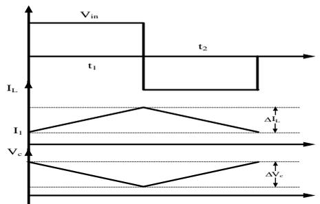
Figure 7. Waveforms Showing Voltage Output with Change in Inductor Current Along with Change in Capacitor Voltage
