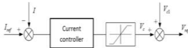
Figure 4. Current control diagram according to Lecocq method
