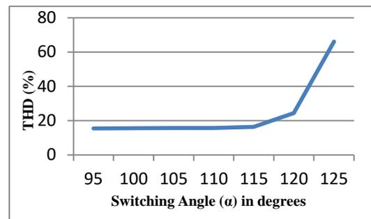
Figure 6(c). Variation of THD with switching angle for three-phase 12-pulse converter
