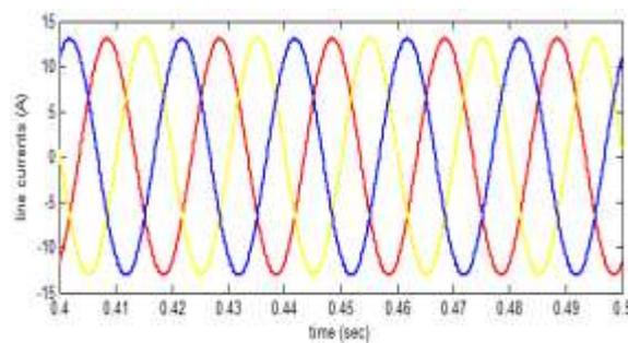
Figure 7(c). line currents for three-phase 12-pulse converter with three-phase harmonic filters
