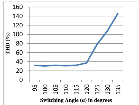
Figure 4(c). Variation of THD with switching angle for three phase 6-pulse converter
