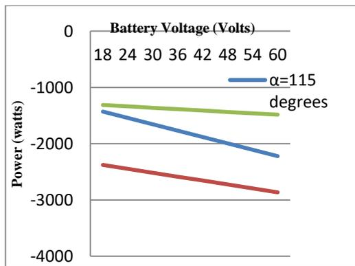
Figure 6(d). Variation of power with battery voltage at different switching angles for three-phase, 12-pulse converter
