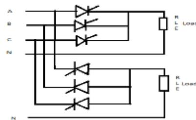
Figure 2. Circuit diagram of two three-phase half-wave 3-pulse ac-to-dc converter
