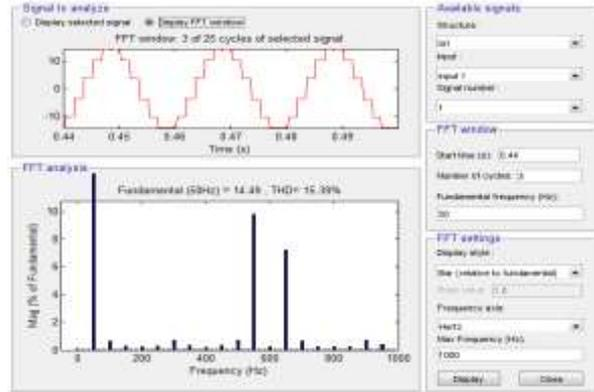
Figure 6(a). Line current with THD and harmonics for three phase 12-pulse converter
