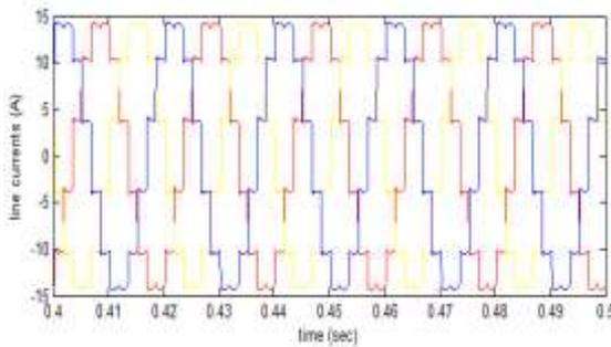
Figure 7(b). Line current for three phase 12- pulse converter
