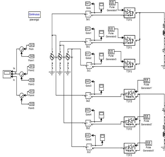
Figure 5. Simulink model of Two three-phase, half-wave, 3-pulse Converter
