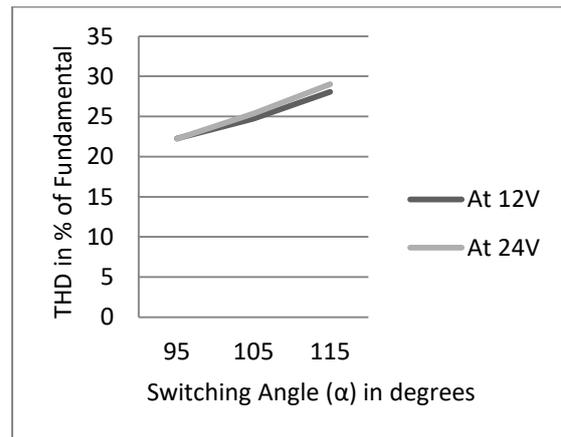
Figure 5(c). Variation of THD with switching angle for two three phase half wave 3-pulse ac to dc converter
