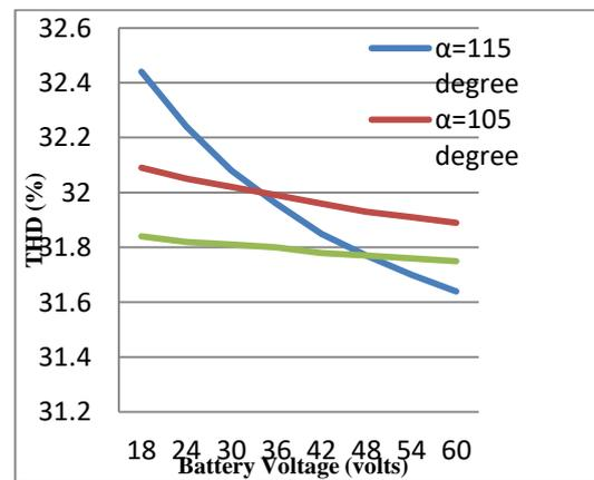
Figure 4(e). Variation of THD with battery voltage at different switching angles for three phase 6-pulse converter
