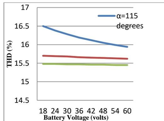
Figure 6(e). Variation of THD with battery voltage at different switching angles for three-phase, 12-pulse converter
