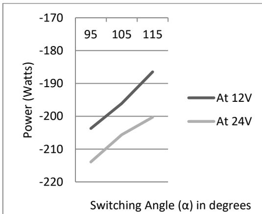
Figure 5(b). Variation of power with switching angle for two three phase half wave 3-pulse ac to dc converter
