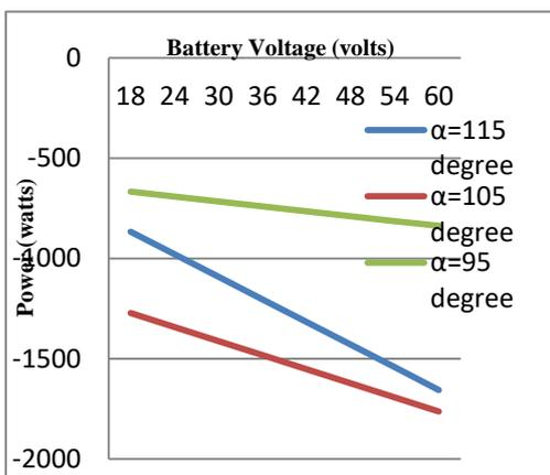
Figure 4(d). Variation of power with battery voltage at different switching angles for three phase 6-pulse converter
