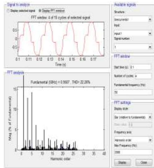
Figure 5(a). Line current with THD and harmonics at switching angle  $\alpha=95^\circ$  for two, three-phase, half-wave 3-pulse converter
