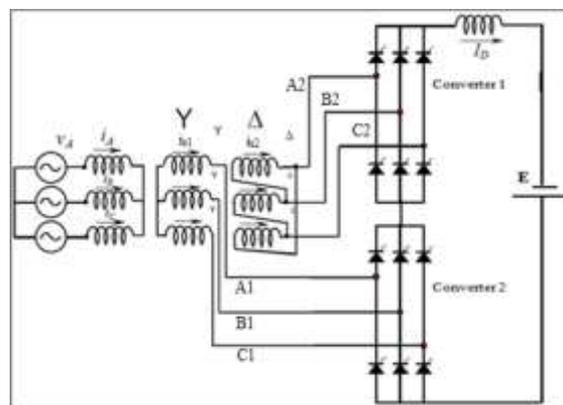
Figure 3. Circuit Diagram of Three-Phase 12-Pulse Converter
