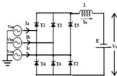
Figure 1. Circuit diagram of three phase 6-pulse converter
