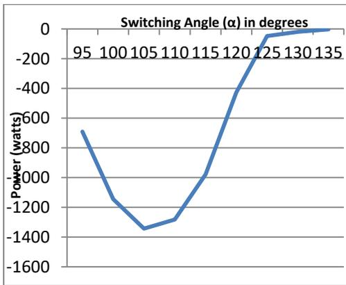
Figure 4(b). Variation of power with switching angle for three phase 6-pulse converter
