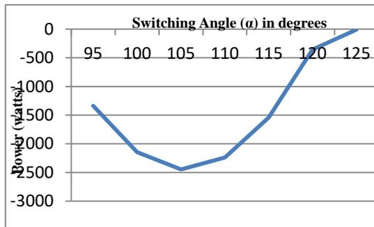
Figure 6(b). Variation of Power with switching angle for three-phase, 12-pulse converter
