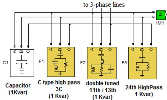
Figure 7. Simulink model of filters
