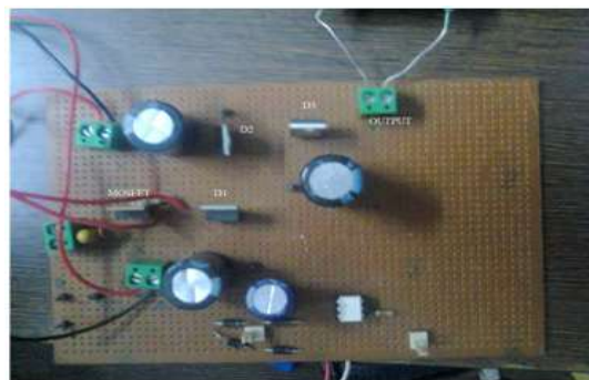
Figure 23. High step-up DC-DC Converter for Photovoltaic Application
