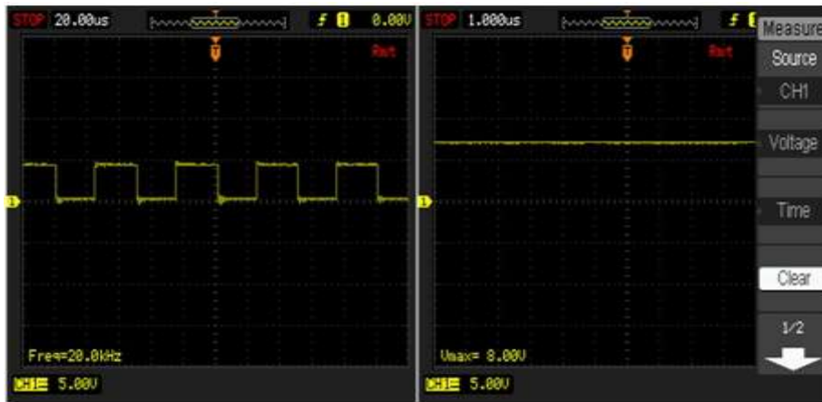
Figure 10. PWM and output voltage waveform of a fixed step size based P&O using DSO
