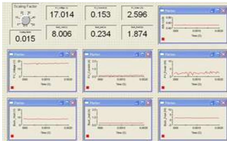
Figure 11. Real time Input & Output Voltage, Current and Power display of a fixed step size based P&O in dSPACE control desk
