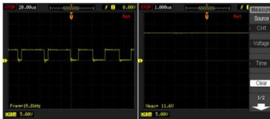
Figure 13. PWM and output voltage waveform of a variable step size based P&O using DSO
