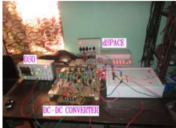
Figure 9. Hardware setup of PV fed Dspace based DC-DC converter
