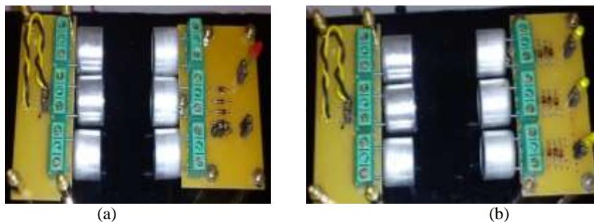
Figure 7. The arrangement of the AET MIMO system where all the receiving transducer connected to the (a) single load and (b) multiple load
