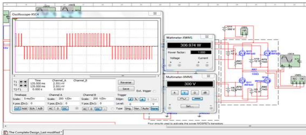
Figure 16. Splitting the PWM Pulses to Two Parts for Drive Circuits
