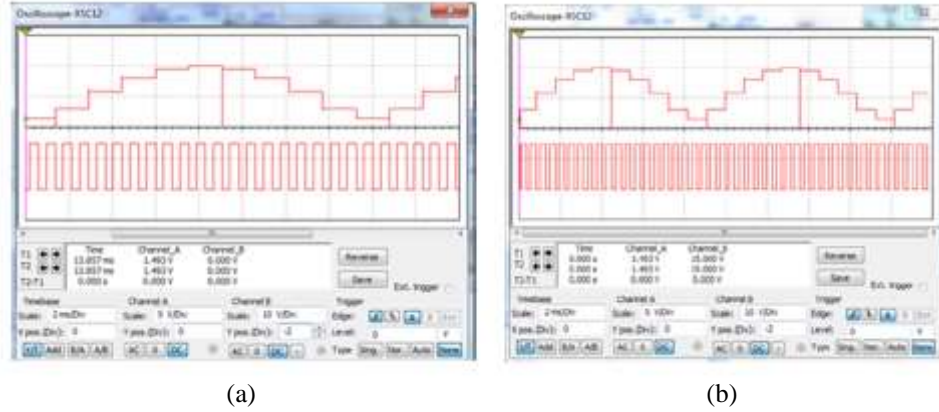
Figure 9. (a) Output Waveform of the Frequency Divider and Reference Signal Generator at Half of Maximum Reference Frequency Value, (b) Output Waveform of the Frequency Divider and Reference Signal Generator at Maximum Reference Frequency Value
