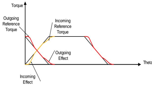
Figure 5. Simple Modification Scheme used to Compensate Torque Error in Phase Torque Control Loop
