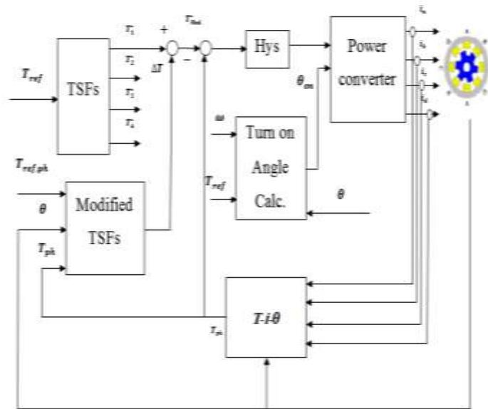
Figure 6. Control Block Diagram of Modified Turn-on Angle Scheme
