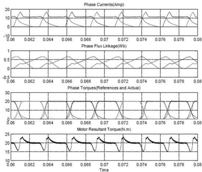
Figure 12. Phase Currents, Flux Linkages, Phase Torques and Motor Resultant Torque for Cosine TSF at Speed 1200 rpm and 20Nm Reference Torque with Turn-on Angle Control Scheme
