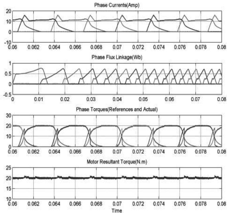
Figure 18. Phase Currents, Flux Linkages, Phase Torques and Motor Resultant Torque for Exponential TSF at Speed 1200 rpm and 20Nm Reference Torque with Modification Rules and Turn-on Angle Control Scheme
