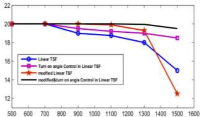
Figure 19. Average Motor Torque Versus Rotor Speed for Different Conditions: Conventional Linear TSF, with Turn-on Angle Control, with Modification Rules and Both Modifications and Turn-on Angle Control Schemes
