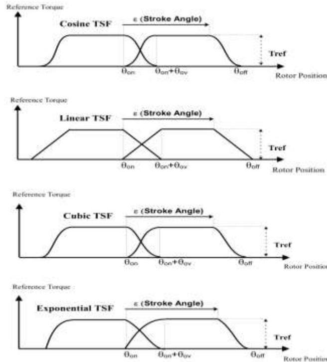
Figure 2. Four conventional TSFs: Cosine, linear, Cubic and exponential types
