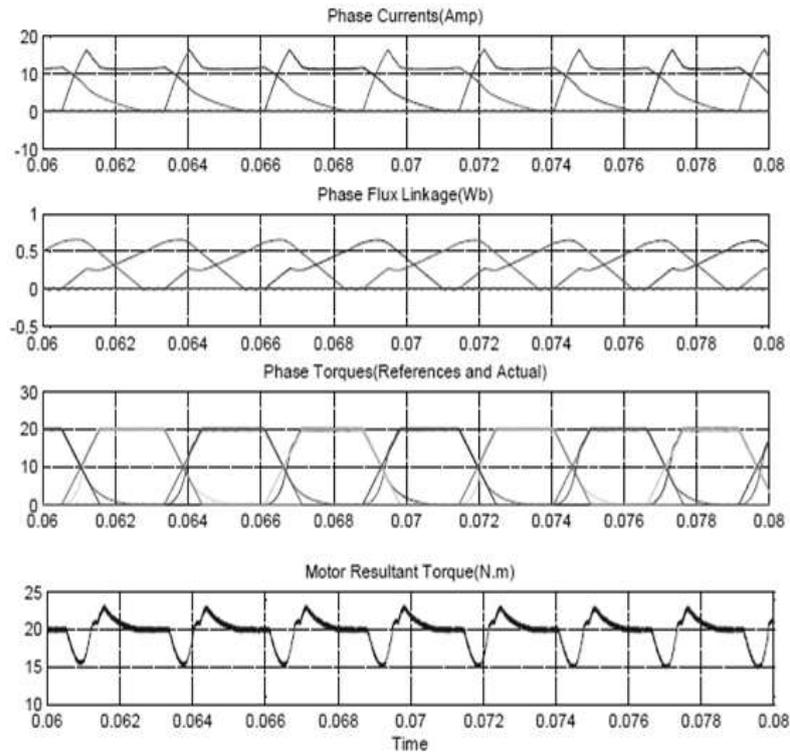
Figure 11. Phase Currents, Flux Linkages, Phase Torques and Motor Resultant Torque for Linear TSF at Speed 1200 rpm and 20Nm Reference Torque with Turn-on Angle Control Scheme
