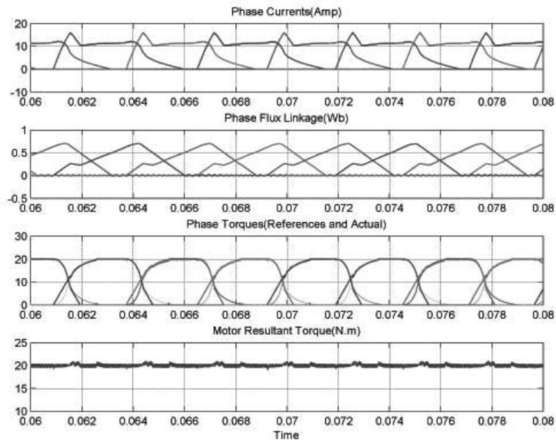
Figure 15. Phase Currents, Flux Linkages, Phase Torques and Motor Resultant Torque for Linear TSF at Speed 1200 rpm and 20Nm Reference Torque with Modification Rules and Turn-on Angle Control Scheme
