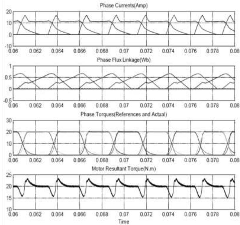
Figure 13. Phase Currents, Flux Linkages, Phase Torques and Motor Resultant Torque for Cubic TSF at Speed 1200 rpm and 20Nm Reference Torque with Turn-on Angle Control Scheme
