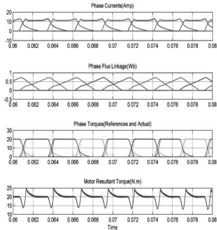
Figure 8. Phase Currents, Flux Linkages, Phase Torques and Motor Resultant Torque for Cosine TSF at Speed 1200 rpm and 20Nm Reference Torque
