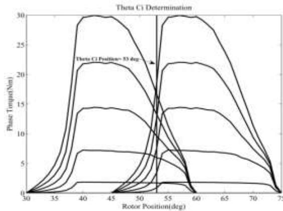
Figure 3.  $\theta_c^i$  Determination for the Considered 4-Phase SRM
