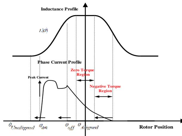
Figure 4. Receding Turn-on Angle Effects on the Shape of Phase Currents
