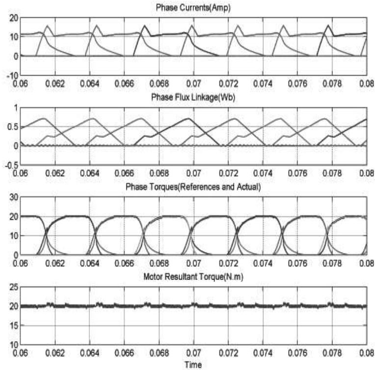
Figure17. Phase Currents, Flux Linkages, Phase Torques and Motor Resultant Torque for Cubic TSF at Speed 1200 rpm and 20Nm Reference Torque with Modification Rules and Turn-on Angle Control Scheme
