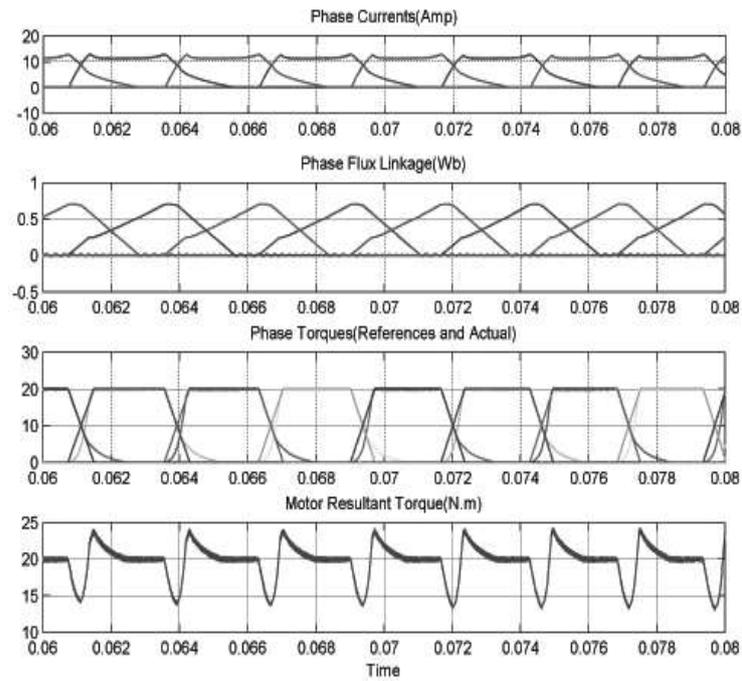
Figure 7. Phase Currents, Flux Linkages, Phase Torques and Motor Resultant Torque for Linear TSF at Speed 1200 rpm and 20Nm Reference Torque
