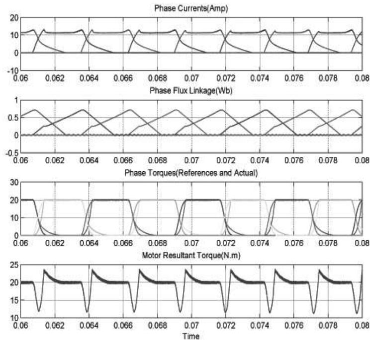
Figure 10. Phase Currents, Flux Linkages, Phase Torques and Motor Resultant Torque for Exponential TSF at Speed 1200 rpm and 20Nm Reference Torque
