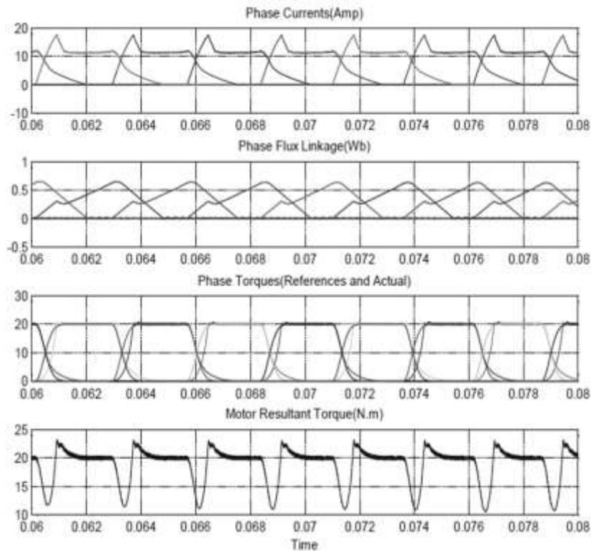
Figure 14. Phase Currents, Flux Linkages, Phase Torques and Motor Resultant Torque for Exponential TSF at Speed 1200 rpm and 20Nm Reference Torque with Turn-on Angle Control Scheme
