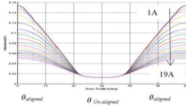
Figure 1. Inductance Profile of Considered 4-Phase SRM Versus Current and Rotor Position Variations
