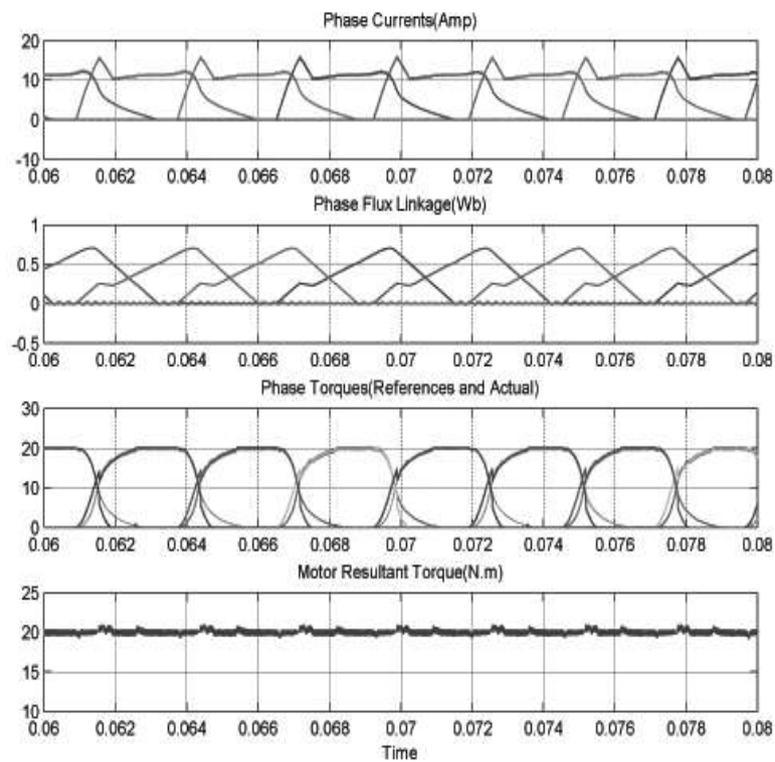
Figure 16. Phase Currents, Flux Linkages, Phase Torques and Motor Resultant Torque for Cosine TSF at Speed 1200 rpm and 20Nm Reference Torque with Modification Rules and Turn-on Angle Control Scheme
