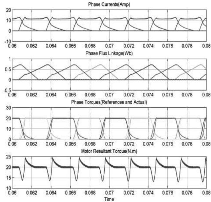
Figure 9. Phase Currents, Flux Linkages, Phase Torques and Motor Resultant Torque for Cubic TSF at Speed 1200 rpm and 20Nm Reference Torque
