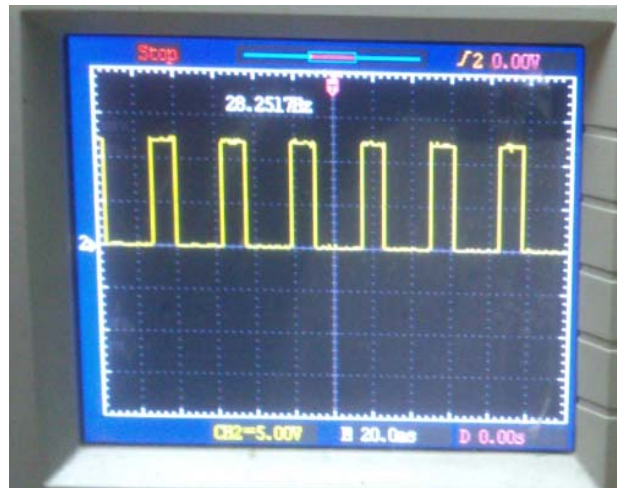
Figure 17. Driver Output Pulse for M5
