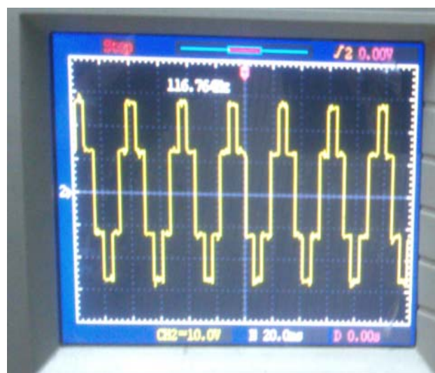
Figure 19. Line to Line Voltage
