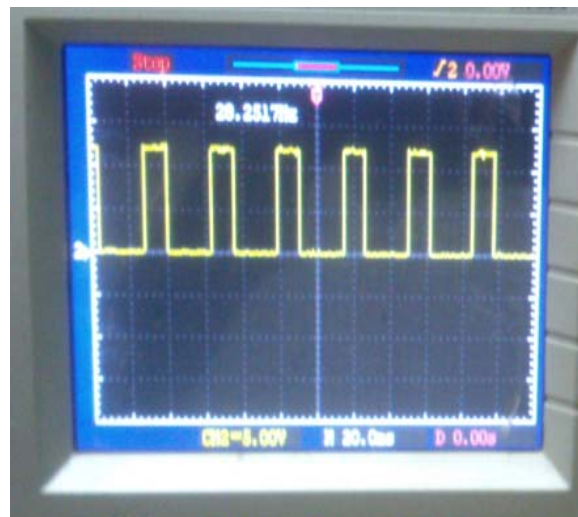
Figure 15. Driver Output Pulse for M1
