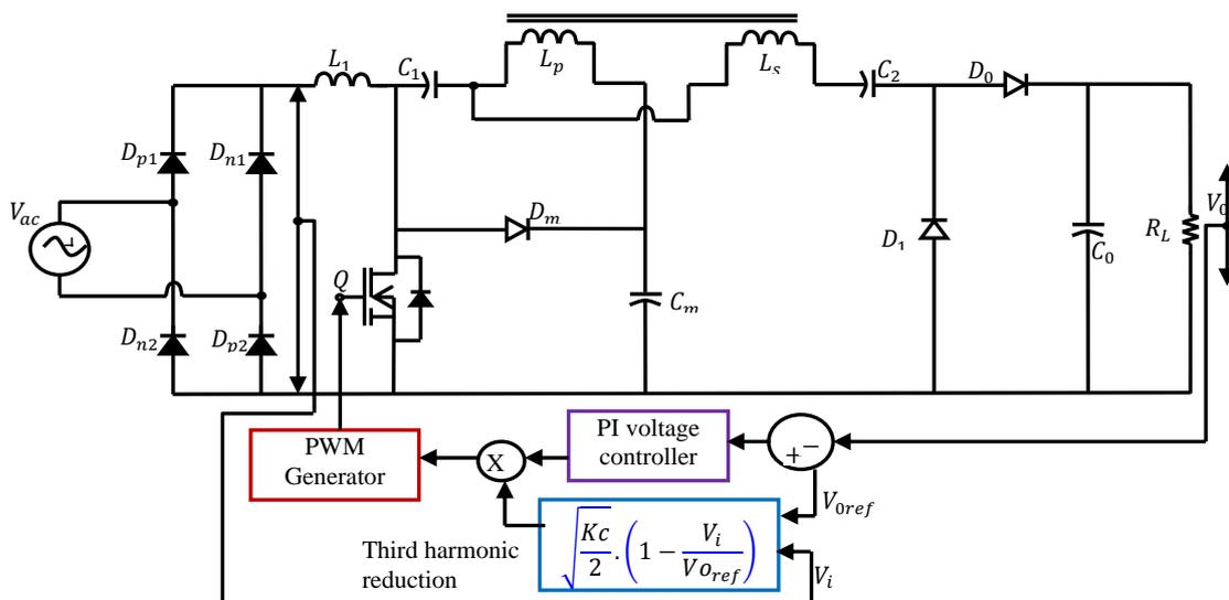
Figure 5. The block diagram of the proposed converter control loop
