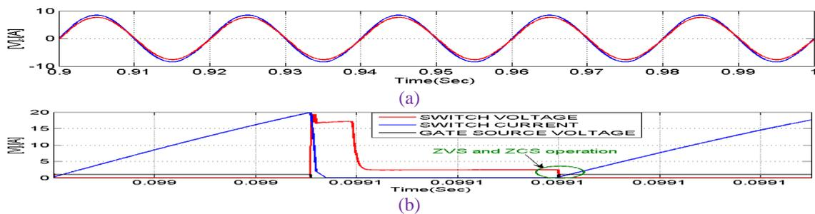
Figure 10. The soft-switching operation of proposed TI-SEPIC-DCM converter
