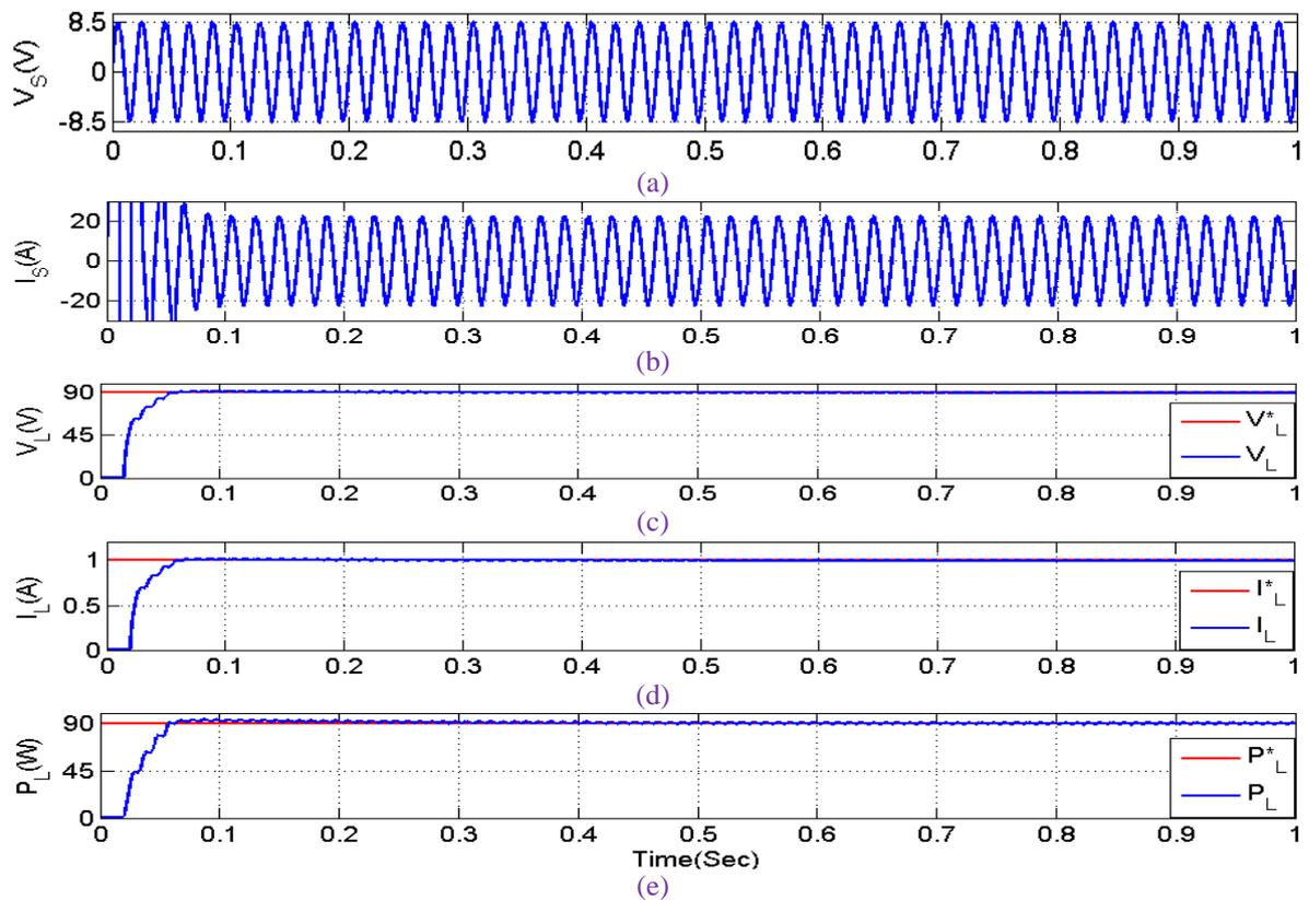
Figure 7(a)-(e). The proposed converter operates at rated supply voltage of (8.48 V)
