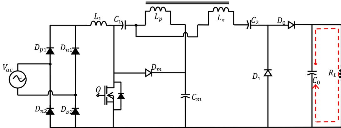
Figures 4(c). The proposed TI-SEPIC- DCM converter operating in DCM presents at Mode 2 operation
