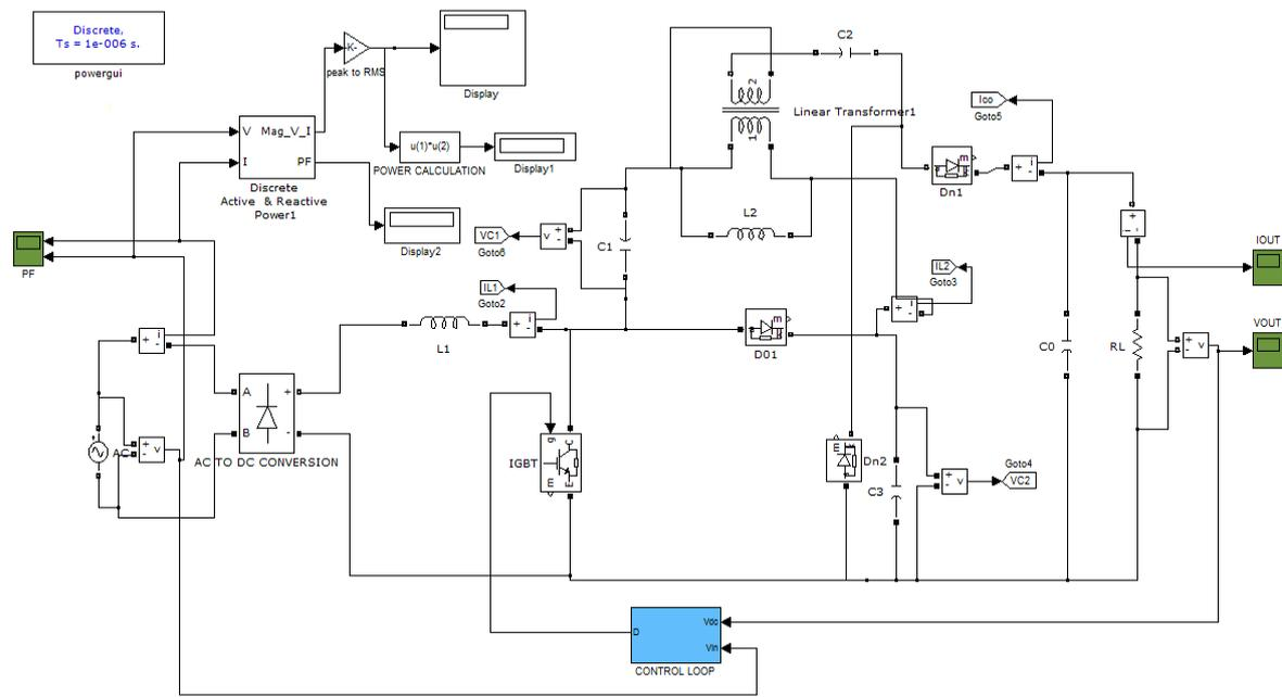
Figure 6. MATLAB/Simulink experimental setup of the proposed TI-SEPIC-DCM converter
