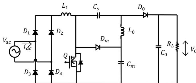
Figure 2. The DCM SEPIC converter
