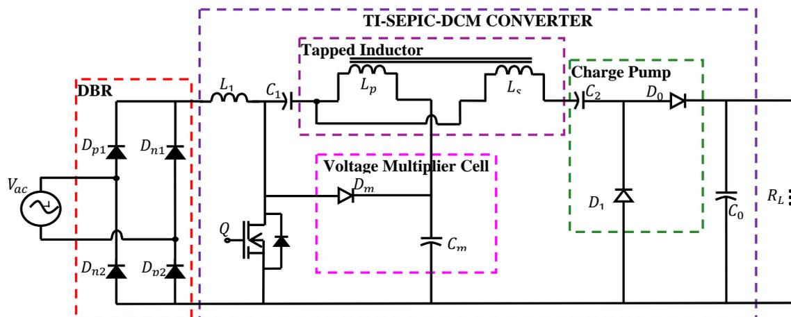
Figure 3. Schematic diagram of the proposed SEPIC converter with the TI model operating in Discontinuous Conduction Mode (TI-SEPIC-DCM)
