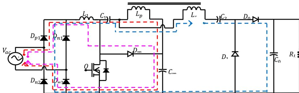
Figures 4(b). The proposed TI-SEPIC- DCM converter operating in DCM presents at Mode 1 operation
