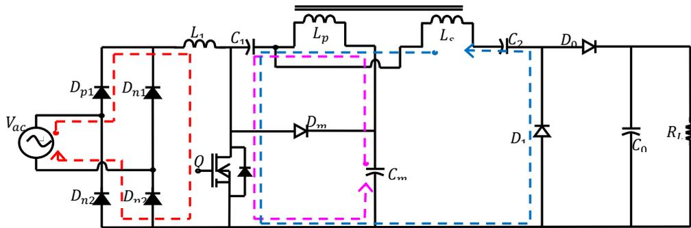
Figures 4(a). The proposed TI-SEPIC- DCM converter operating in DCM presents at Mode 0 operation
