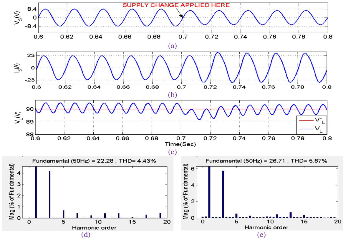
Figure 8(a -e). The dynamic performance of the proposed converter during a step change
