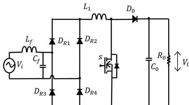
Figure 1. The conventional boost preregulator functioning in DCM
