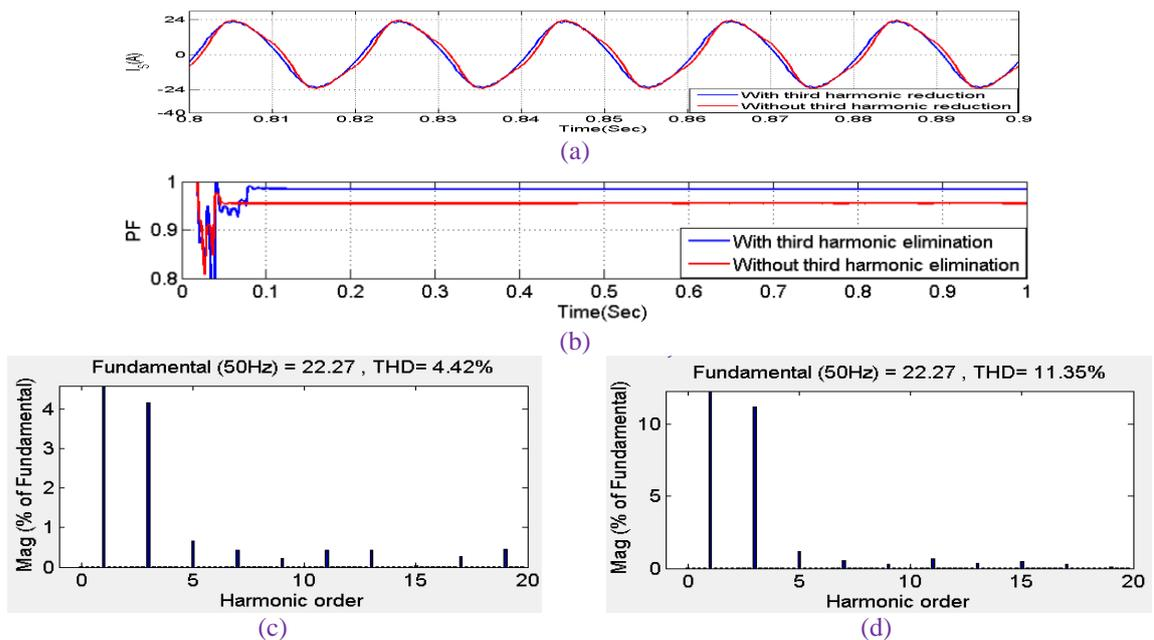
Figure 9. The proposed TI-SEPIC-DCM converter performance is compared with and without the implementation of the third-harmonic reduction technique
